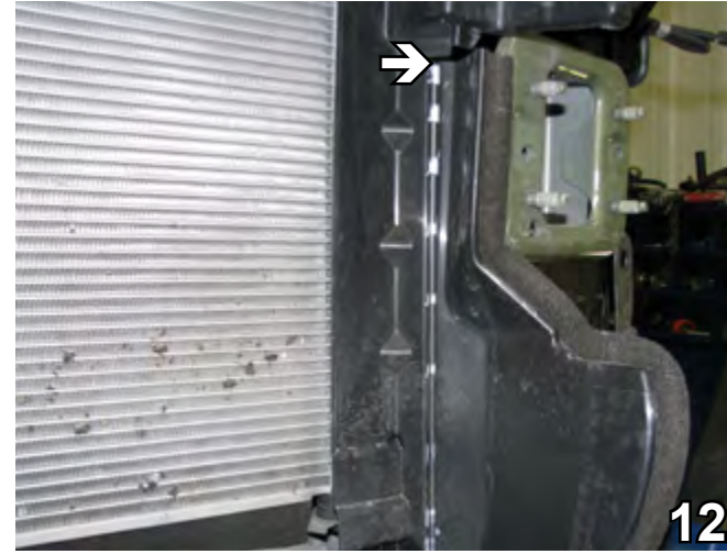
12. On the driver's side using the utility knife, cut down the air dam at the slit. Remove the cut portion of the air dam.
