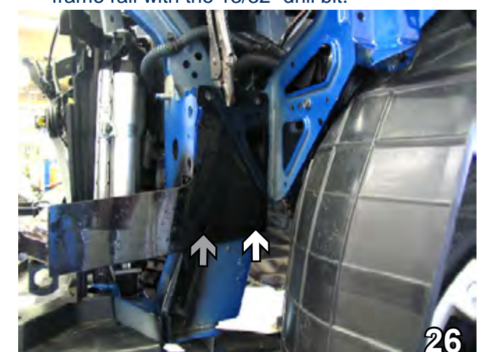
26. On the driver's side, insert one 3/8-16 nut plate through frame opening and align to lower front hole. Install 3/8-16 x 1 1/4" bolt with 3/8" lock washer and tighten (see grey arrow). Install 3/8-16 x 1 1/4" bolt to lower back hole (see white arrow) with three 3/8" flat washers, 3/8" lock washer and 3/8-16 hex nut and tighten. In upper holes, install 3/8-16 x 1 1/4" bolts with 3/8" lock washers, 3/8-16 hex nuts and tighten to specs.
