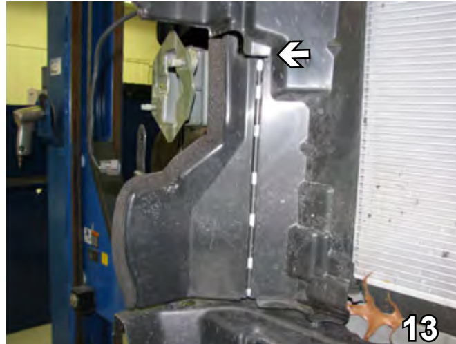
13. On the passenger's side, using the utility knife, cut down the air dam at the slit. Remove the cut portion of the air dam.
