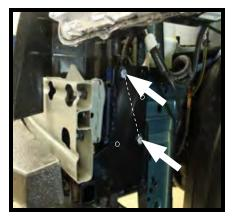
8. Slide the baseplate downward at a slight angle and then up so the baseplate frame runs parallel with the vehicle's main frame. The top of the baseplate endplate should be flush with the top of frame. The back edge of the baseplate endplate should be aligned with the front edge of the main frame.
