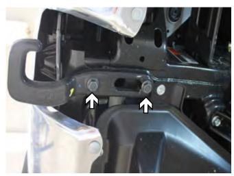
Using a 17MM socket, remove the two
