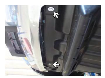
Using a 12MM socket, remove the front two (2) bolts from the belly pan and remove from the vehicle.
