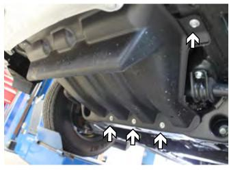
Using a 12MM socket, remove the three
