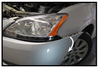
5. Pull the corners of the fascia out and forward to unclip. Remove the fascia from the vehicle and set aside.
