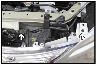
2. Remove the four (4) push pins from the top edge of the fascia. There are two (2) on each side.
