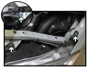
Using a 10MM socket, remove the two
