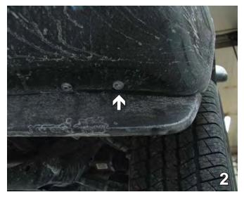
2. Using a 10MM socket, remove one metric bolt from the front of the fascia. Set bolt aside to be reinstalled later. Do this to both sides of the vehicle.
