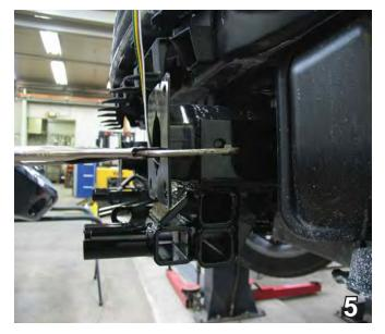
5. Lift baseplate straight up and slide forward up to dimple in frame. Baseplate should be straight and clamped into place with vise grips.
