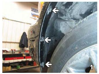
Using a 10MM socket, remove three metric bolts just forward the front tire, on the wheel well. Once bolts are removed from the wheel well, pull plastic back and remove two metric bolts with a 10MM socket. Set bolts aside to be reinstalled later. Do this to both sides of the vehicle.
