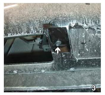
Using a 10MM socket, remove one metric bolt located on the side of the opening in the fascia. Set bolt aside to be reinstalled later. Do this to both sides of the vehicle.
