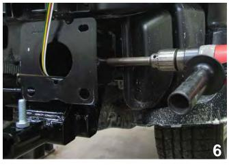
6. Using the baseplate as a template, drill two holes into the side of the frame and one hole in the bottom of the frame with a 17/32" drill bit. Place a piece of tubing over drill bit for protection while drilling out holes. Insert the 1/2" nut plates into the frame and align with drilled holes. Insert a 1/2-13X1 1/2" hex bolt and 1/2" lock washer into each hole and tighten down with a 3/4" socket. Do this to both sides of the vehicle.
