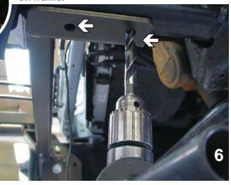
While holding bumper brackets in place align baseplate to the interior hole and insert 1/2-13 x 4" bolts and flat washers on both sides. before tightening, adjust bumper bracket to the previous height, then slide baseplate up to the bottom of the frame and tighten bolt and hex nuts.
