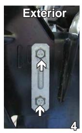
3. Using an 18MM socket, remove three bolts from behind the bumper - two on the bottom, one on the top. Do to both sides and set bolts and bumper aside for later reinstallation.
