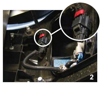
Located behind the pumper is a red cap on plug. Slide red cap up then push in to release plug, set plug up out of the way.
