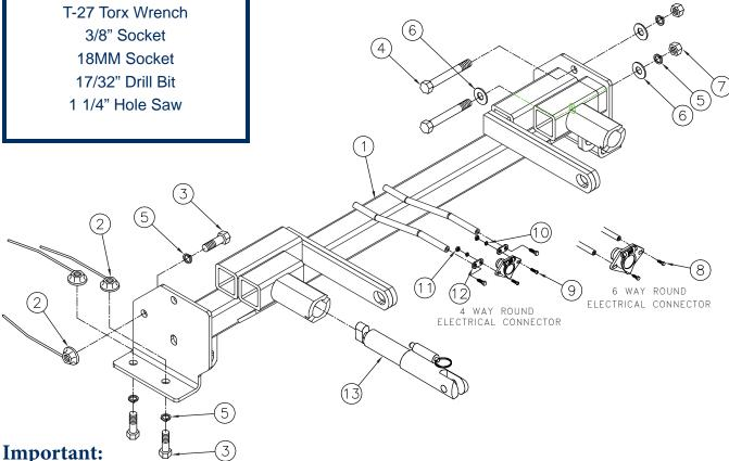
Use only genuine factory replacement parts on your baseplate. Do NOT substitute homemade or non-typical parts. If a bolt is lost or in need of replacement, for your safety and the preservation of your baseplate, be sure to use a replacement bolt of the same grade (In most cases it will be Grade 5, please reference the parts list above). Replacement parts may be ordered through your nearest Blue Ox® Dealer or Distributor.
