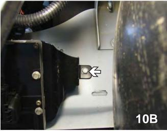
10. On the driver's side, using a 10MM socket remove two bolts on the front and one on the back then let the computer hang down in order to do drilling. Set bolts aside to be reinstalled later.
