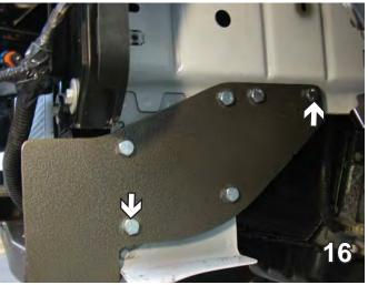
16. On the driver's side, mount the baseplate using 3/8" x 1 1/4" hex bolts going in and 3/8" lock washers and 3/8" hex nuts. Be sure to use LOCTITE Red on ALL bolts.
