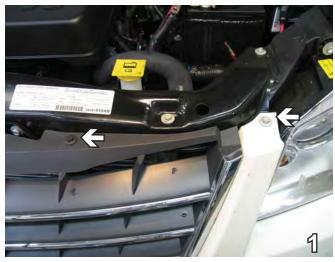
Using a 10MM socket remove the bolt above the headlight. Using a flat screwdriver remove the push pin. Do this to both sides and set bolts and push pins aside for later reinstallation.
