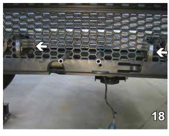
18. Hold the plastic shield up to the front and with the utility knife cut out as needed for the baseplate tabs.
