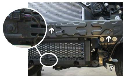
Using a flat screwdriver, remove the push pin from the air temperature control and let it hang (see arrow in inset). Continue removing four more push pins across the top. Remove the plastic cover.
