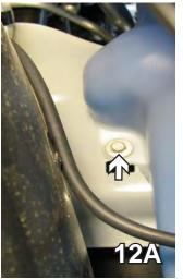
12. Using a 10MM socket, remove the two bolts one on each side of the washer reservoir. Set washer reservoir and bolts aside to be reinstalled later.
