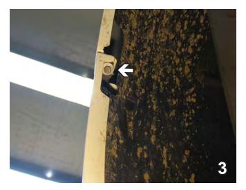
3. Continuing just forward of the front tire on the wheel well, using an 10MM socket, remove the bolt in the corner. Do to both sides and set bolt aside for later reinstallation.
