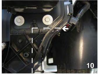
10. Using a utility knife, cut straight across right along side the bottom of the plate and straight up to a 90° angle. Do this on both sides.
