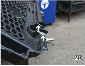
20. On the back side of the plastic shield, cut off the six tabs.
