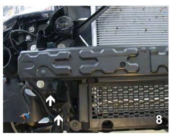
8. Using a flat screwdriver, remove the push pin. Then using a utility knife, cut the loose plastic right along the bumper. Do this to both sides.
