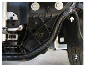
9. On the driver's side, pull out the push pin clip and take the wire harness out.
