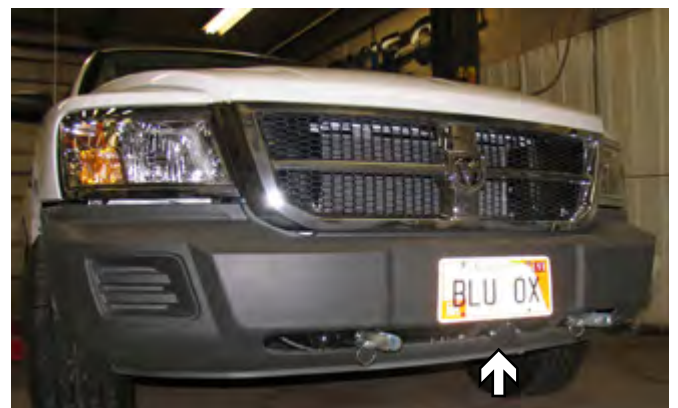
Possible location for the electrical bracket
