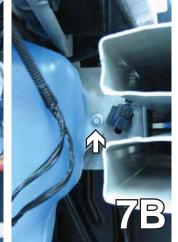
On the passenger side, using a 10MM socket, remove the three bolts holding the washer reservoir. Unplug the wires (gray arrow) and plug the water line. Set aside to be reinstalled later.
