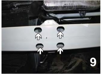
To remove the bumper, using a 13MM socket, remove the four bolts. Do this to both sides.
