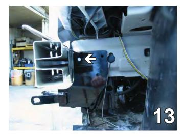
13. Slide the baseplate up from underneath, line up with the drilled hole. Make sure the baseplate is straight and clamp. Using the baseplate as a template, drill the remaining three holes with the 13/32" drill bit.
