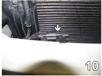
10. On the back side of the bumper, unplug the air temperature control. Remember to replug after the bumper is reinstalled.
