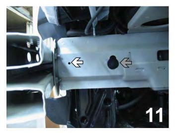
11. On the driver's side, with a 1 1/4" hole saw, drill a hole with the back existing hole to insert the wire nut for baseplate installation. Use the 13/32" drill bit to enlarge the existing hole (white arrow) as a starting point.
