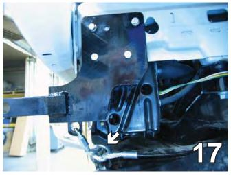
17. Attach the baseplate safety cables. Position the cables around a solid piece of the frame.
