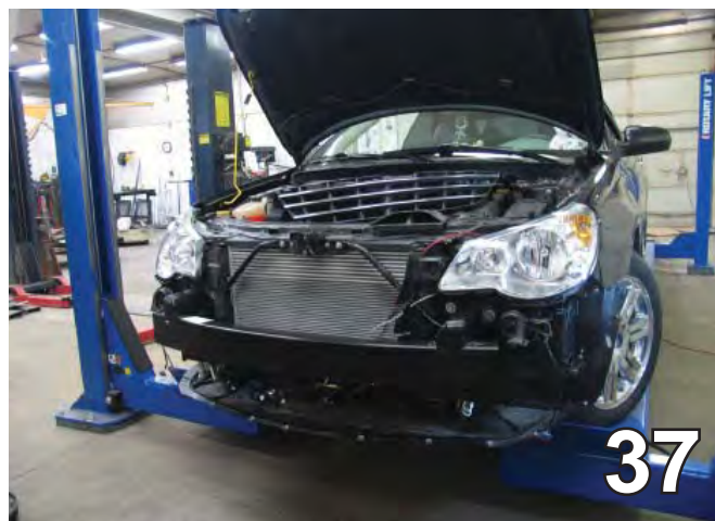
37. Reinstall the headlight assembly, reconnect the transmission coolant line, reconnect the sensor, replug the running lights, reinstall the fascia and the grille.
