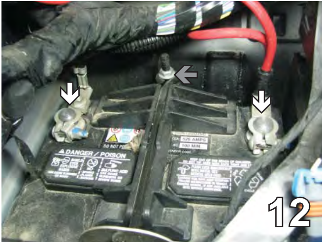
12. On the driver's side, use a 10MM socket to remove the two bolts on the sides (white arrows). Use a 13MM socket to take the nut off the back (gray arrow). Slide the battery out the side and set aside to be reinstalled later.
