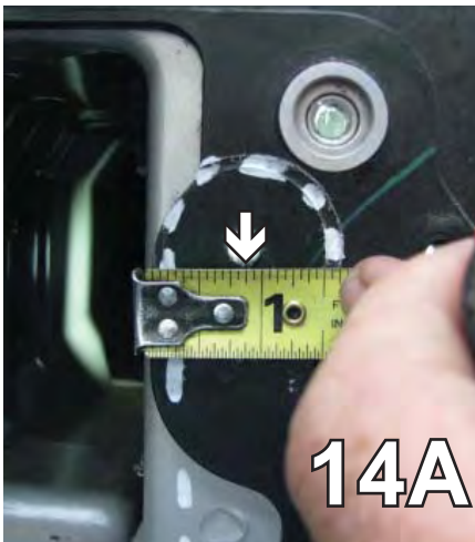
14A. Saw out a slot by first measuring 7/8" in from the inside. Using a 1 1/4" hole saw, drill where the bumper bolts were on both ends. Use a reciprocating saw to connect the cuts. Do this on both sides.
