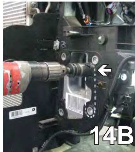
14A. Saw out a slot by first measuring 7/8" in from the inside. Using a 1 1/4" hole saw, drill where the bumper bolts were on both ends. Use a reciprocating saw to connect the cuts. Do this on both sides.
