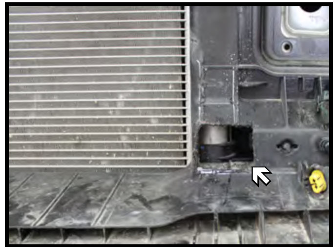
29. Trimming of the air dam is required for the placement of the permanent baseplate safety cables. Loosely attach the baseplate at the upper front bolt location. Mark the area on the air dam just behind the convenience link (25A white arrow). Remove the baseplate and cut a hole in the air dam to allow the connection of cables/quicklinks to baseplate (25B). Be aware of radiator condenser and other related items behind the plastic.
