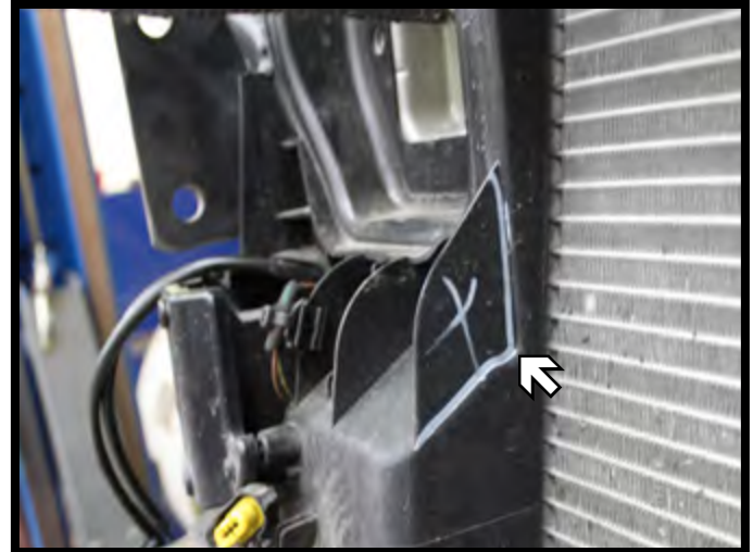
28. On the passenger side, trim off the tab using the outer edge as a guide.
