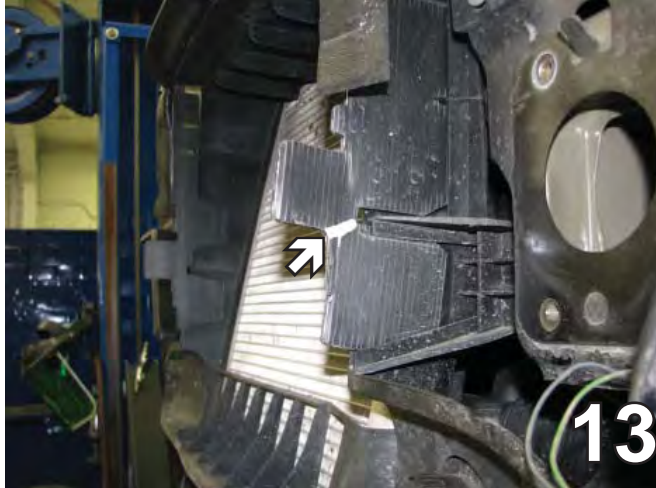
13. Using a utility knife, trim the tab as shown. Do this on both sides.
