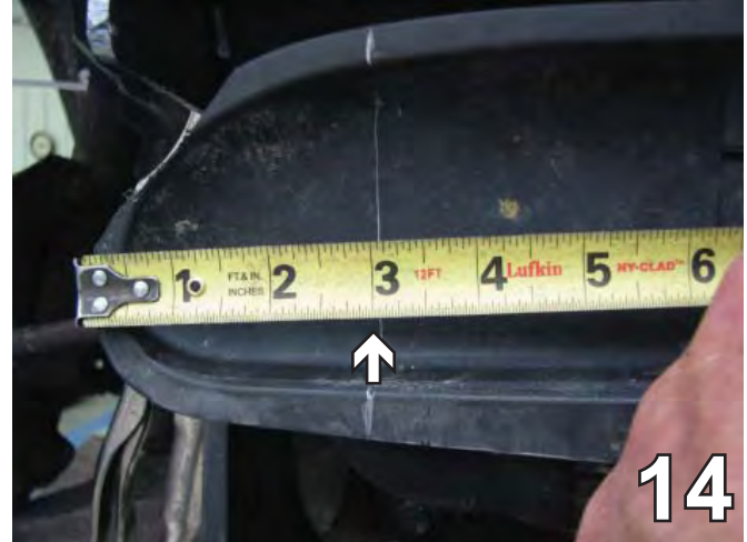
14. On the driver's side, disconnect the temperature sensor. It will need to be relocated. Cut straight down along the edge of the plug plate. On the passenger side, measure 3" over from the end of the frame and cut straight down.
