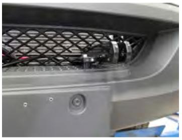
18. Use 3/4" spacertube before installing 8MM-1.25 x 50MM bolt and 8MM lockwasher, typical both sides.
