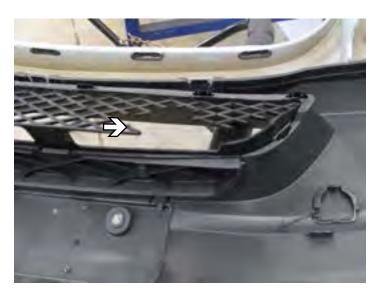
17. Hold front facia up to frame and mark to cut out for clearance around baseplate. After cutting suffient amount for clearance, re-attach facia to vehicle.
