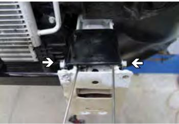
14. On inner frame hole (left) use a 3/8"x1-1/2" bolt, 3/8" lock washer and 3/8"-16 whiz nut. On outer frame (right) use a 3/8"x1-1/4" bolt, 3/8" lock washer and 3/8"-16 whiznut. Repeat on passenger side.
