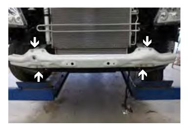
11. Remove the eight (8) bolts using a 13mm socket to remove bumper from frame.
