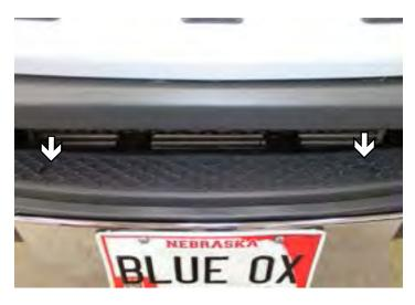
5. Remove the two (2) screws above the license plate bracket using a 25 Torx.
