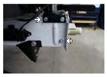
15. After upper front bolts are tighten down continue drilling upper back and lower front holes. In upper back hole (top) use 3/8"x4" bolt, 3/8" lockwasher and 3/8"-16 whiz nut with nut on inner side of frame. On front lower hole (bottom) use 3/8"x4" bolt and nylon lock nut with nut on outer side of frame.
