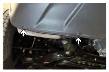
At the front of vehicle on the underside of facia using a straight screwdriver, turn the two (2) facia pins 90 degrees to unlock and remove. Both driver and passenger sides.
