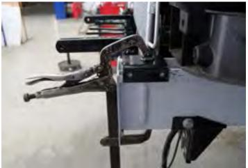
12. Securely clamp the baseplate in place to frame using Large Vise-Grips on both sides of vehicle.
