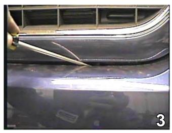
There is a slot under each headlight and three under the grille assembly that join the bumper fascia. Insert a flat head screw driver and pry down while pulling the fascia forward. Set the headlight assemble aside to be reinstalled later.
