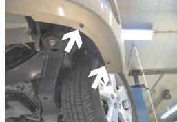
6. Remove the two phillips screws just forward of the front tire, on lower edge of fascia with the phillips screw driver, on both sides.
