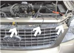
**2.** Remove the six push pins from the top edge of fascia between headlight assemblies, the driver's side shown.
