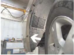
**3.** Remove the two phillips screws just forward of the front tire, on fascia and wheel well edge with the phillips screw driver, on both sides.
