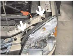
**4.** Pull the two clips straight up just behind headlight assembly, pull forward, unplug electrical and set aside, on both sides.
