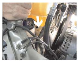
**9.** Using the 8MM socket, remove two metric bolts from radiator reservoir on the passenger side of engine compartment and pull unit away from side wall. Remove the metric bolt on the side wall and just under radiator reservoir with the 8MM socket.
