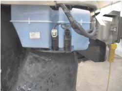
**10.** Remove the metric bolt from washer reservoir on the edge of frame webbing with the 8MM socket on the passenger's side, unplug electrical and fluid line, pull reservoir down and set reservoir aside.
