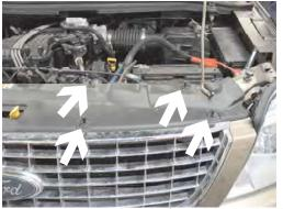
1. Remove the eight push pins from black plastic cover on top side of fascia, the driver's side shown, lift cover and set aside.
