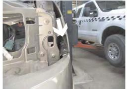
Just behind headlight assembly inside fender and fascia's corner are two metric bolts to remove with the 7MM socket, on both sides.
