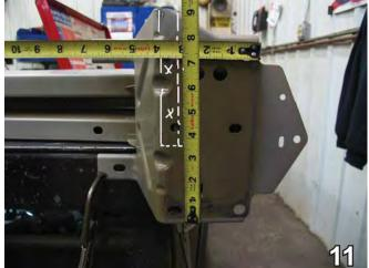
11. Remove the plastic from the front of the metal bumper by releasing the plastic from the slotted clips. On the back side of the metal bumper bracket, measure and mark a rectangle, 3 3/4" from the top of the bumper bracket 3 1/4" in from the outside edge of the bumper and 3/4" wide. *Note: To make cutting easier, flip the metal bumper over as shown in the photo above.* Driver's side is shown in the photo.
