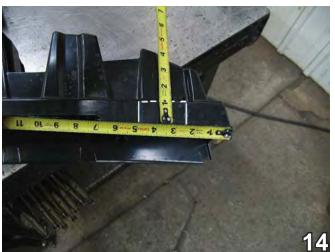
14. On the bottom side of the bumper plastic, measure and mark a rectangle 2 1/2" wide on the raised molding 2 1/4" from the outside edge of the plastic and 1 1/4" high. Trim away the area with the utility knife to open for baseplate installation. Do this to both sides of the plastic. Driver's side is shown in the photo
