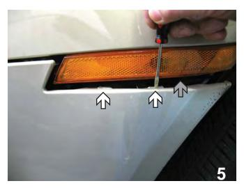
5. Pull out on the fascia corner, below the turn signal marker. Using a small flat screwdriver, push up to release one clip under the turn signal (see grey arrow. Release two tabs under the turn signal (see white arrows)
