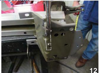
12. Using the reciprocating saw, start both vertical cuts and continue until reaching the top side of the bumper bracket support. Using the vise grips, bend the cut metal back and forth until it pulls away.Do this to both sides of the metal bumper. Driver's side is shown in the photo.
