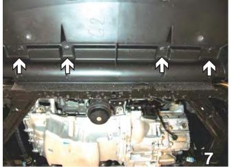
7. Remove four pushpins from the bottom of the bellypan. Pull belly pan down to remove.Set pushpins and belly pan aside to be reinstalled later.
