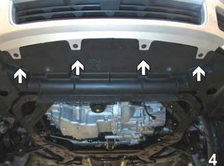
4. Using the 7mm socket, remove four metric bolts from underneath the center of the fascia. Set bolts aside to be reinstalled later.
