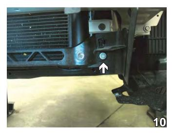
10. Using the 10mm socket, remove the metric bolt securing the air dam to the radiator support. Do this to both sides of the vehicle. Discard the bolts and air dams as they will not be reinstalled.
