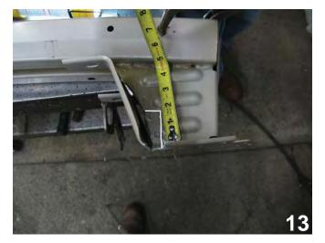
13. Using the reciprocating saw, cut from the outside edge of the bumper bracket's vertical cut, toward the front of the bumper 2" and then across to the inside edge of bumper bracket. Cut along the bumper bracket support contour to the bumper bracket. Finally, complete cutting the rectangular area shown in step 12. Do this to both sides of the metal bumper. Driver's side is shown in the photo.
