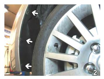
2. Just forward of the front tire, inside the wheel well, remove three pushpins. Do this to both sides of the vehicle. Set pushpins aside to be reinstalled later.
