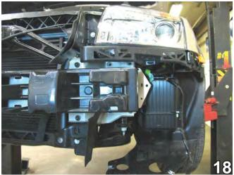
18. Reinstall the metal bumper. Install only two bolts on each side to hold the bumper in place because it will be removed again. It is not necessary to insert the plastic to the front of the bumper at this time.
