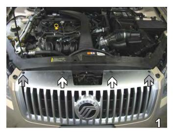
Using the 10mm socket, remove two metric bolts from the top corners of the grille (see grey arrows). Remove two pushpins from the top of the grille (see white arrows). Set pushpins and bolts aside to be reinstalled later.
