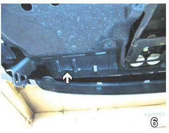
On the front corner of belly pan, use the 10mm socket to remove one metric bolt. Do this to both sides of the vehicle. Set bolts aside to be reinstalled later.
