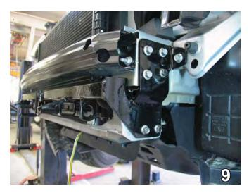
Align baseplate with the seven existing holes in the frame. Insert the existing bolts into the baseplate and tighten. Do this to both sides of the vehicle.
