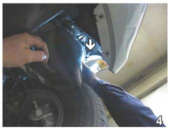
Remove one pushpin from bottom corner of fascia. Do this to both sides of the vehicle. Set pushpins aside to be reinstalled later.
