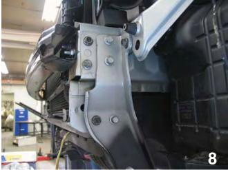
8. Using the 13mm socket, remove seven metric bolts from the frame and tie down bracket. Remove tie down bracket. Do this to both sides of the vehicle. Set bolts aside to be reinstalled later. NOTE: Tie down bracket is not reinstalled, set aside to be returned to the customer.
