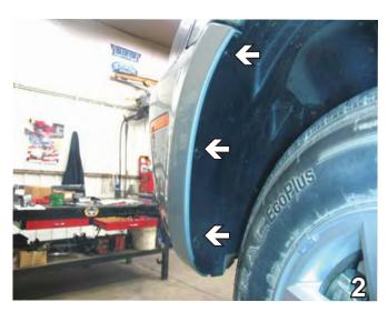
2. Just forward of the front tire, inside the wheel well, remove three Phillips pushpins. Do this to both sides of the vehicle. Set pushpins aside to be reinstalled later.
