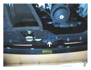
On the front center of belly pan, use the 10mm socket to remove one metric bolt. Pull belly pan down to remove. Set bolt and belly pan aside to be reinstalled later.
