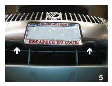
Under the front of fascia, remove a Phillips pushpin on each side of the license plate. Pull fascia forward to remove. Set pushpins and fascia aside carefully to be reinstalled later.
