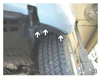
Using the 10mm socket, remove two metric bolts from bottom corner of fascia, just forward of front tire, and one metric bolt just behind the tie down bracket. Do this to both sides of the vehicle. Set bolts aside to be reinstalled later.
