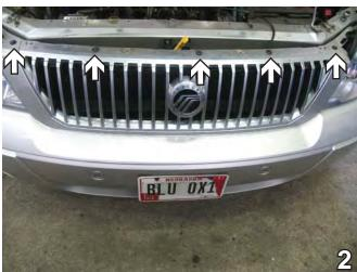
Remove five pushpins from the top of the grille. Set pushpins aside to be reinstalled later.
