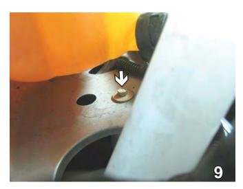
On the bottom of the passenger's side fenderwell, use the 8mm socket to remove one metric bolt. Set bolt aside to be reinstalled later.
