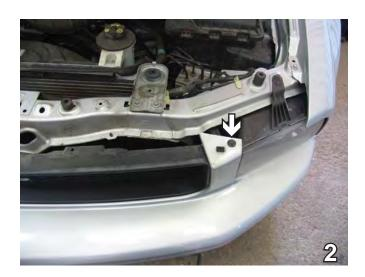
Using the 10mm socket, remove one metric bolt from the top of fascia, next to the headlight assembly. Do this to both sides of the vehicle. Set bolts aside to be reinstalled later.
