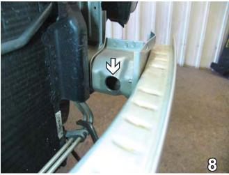
8. Using the 1 1/4" hole saw, drill a hole on the inside edge of frame rail. Do this to both sides of the vehicle. Reinstall metal bumper.
