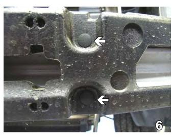
Remove two Christmas tree pushpins from front of styrofoam bumper. Do this to both sides of the vehicle. Pull styrofoam bumper forward to remove. Set styrofoam bumper and pushpins aside to be reinstalled later.
