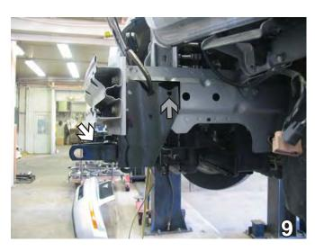
9. Slide baseplate onto the outside of frame rails. Align with upper, existing bolt hole (see grey arrow). The top of the cross tube should be 2 1/4" from the bottom of metal bumper (see white arrow) and the front of baseplate endplate should be resting against the back of the metal bumper bracket. Clamp into place using the vise grips. Do this to both sides of the vehicle.
