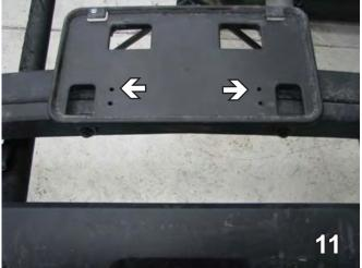
Turn the license plate bracket upside down. Reattach to the bracket, using 1 3/8" self tapping screws. The bottom holes are used to attach the license plate.
