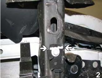
2. Underneath in front of the frame using a hack saw blade, cut 3/8" off of the plastic shield for the radiator. Get as close to the flat washer as possible. Do this on both sides of the vehicle.
