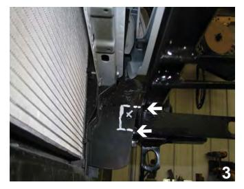
3. Hold the baseplate up to the air dam mark the area width and depth, about 1 1/2", needing to be removed. Cut out the area, snap the lower push pin in place. Do this to both sides of the vehicle.
