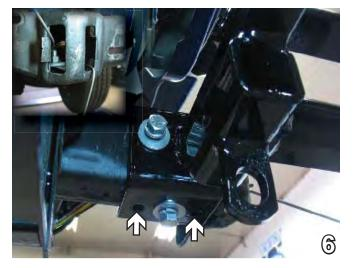
6. Using the baseplate as a template, drill the remaining two holes into the bottom of the frame rail using the 17/32" drill bit. Note: A smaller drill bit may be used to start the pilot hole. Insert 1/2-13 whiz nuts through frame end hole and align to drilled holes. Install 1/2-13 x 1 3/4" hex bolts with 1/2" flat washers and 1/2" lock washers and tighten. Do this to both sides of the vehicle. Insure nut plates are placed lengthwise across frame (see inset) so they do not block other holes.
