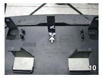
10. Turn the fascia over so that the front is up, lift off the license bracket. Turn the license bracket over. Cut off the single tube in the middle using a hack saw blade.
