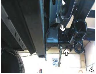
4. Align baseplate to existing holes on bottom and inside of frame rail. Using the vise grips, clamp into place. Do this to both sides of the vehicle.
