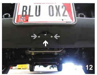
12. Using a 1" hole saw, drill a hole through the bottom of the fascia (see white arrow). Insert electrical connector. Using the electrical connector as a template, drill two holes into the fascia using the 9/32" drill bit. Install 1/4-20 x 3/4" hex bolt with 1/4" flat washer and 1/4" lock washer and 1/4-20 hex nut and tighten.
