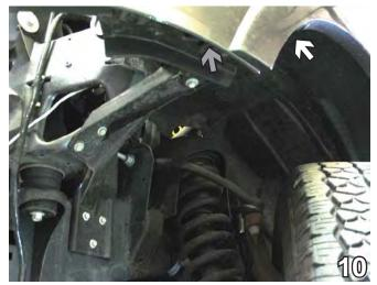
Pull on outer fascia trim (see white arrow) to separate it from the bumper. Pull bumper (see grey arrow) down and then forward to remove. Set bumper and metal bumper aside to be reinstalled later.
