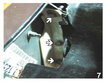
Under the fender, on fascia corner, remove three metric bolts using the 8mm socket. Do this to both sides of the vehicle. Set bolts aside to be reinstalled later.
