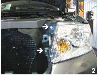
Using the 10mm socket, remove two metric bolts from inside edge of headlight assembly (see white arrows). Raise the clip on upper corner of headlight assembly (see grey arrow). Pull headlight assembly forward to remove (releasing it from two clips behind assembly). Disconnect wiring. Do this to both sides of the vehicle. Set bolts and headlight assemblies aside to be reinstalled later.
