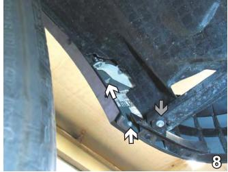
Using the 8mm socket, remove two metric hex nuts from the bottom corner of fascia (see white arrows). Using the 10mm socket, remove one metric bolt from the fascia extension (see grey arrow). Do this to both sides of the vehicle. Set nuts and bolts aside to be reinstalled later.
