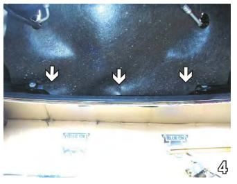
4. Remove three pushpins from metal bumper's lower edge and push air dam out of the way. Set pushpins aside to be reinstalled later.
