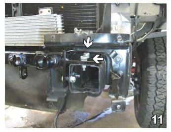
11. Slide baseplate on top of frame rail and align to end of frame rail. Clamp in place with the vise grips. Using the baseplate as a template, drill two holes in the top and side of frame rail using the 17/32" drill bit. On top, install the  $1/2-13 \times 1 \ 1/2$ " bolts with 1/2" lock washers and 1/2-13 hex nuts and tighten. Do this to both sides of the vehicle.
