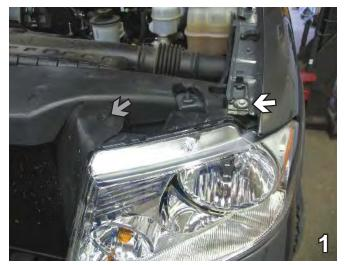
Using the 10mm socket, remove one metric bolt on the upper corner of headlight assembly (see white arrow). Remove one pushpin from the air dam on top of the headlight assembly. Move air dam aside. Do this to both sides of the vehicle. Set bolts and pushpins aside to be reinstalled later.
