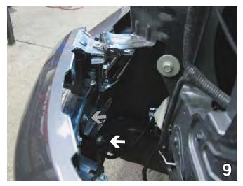
Note: When removing metric bolts from behind the metal bumper, hold bumper securely as it is very heavy. Using the 21mm socket remove lower metric bolt (see white arrow). Using the 10mm socket, remove upper metric bolt (see grey arrow). Disconnect fog lights if necessary. Do this to both sides of the vehicle. Set bolts aside to be reinstalled later.
