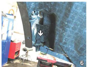
6. Remove one pushpin, just forward of the front tire, on the fender well. Do this to both sides of the vehicle. Set pushpins aside to be reinstalled later.
