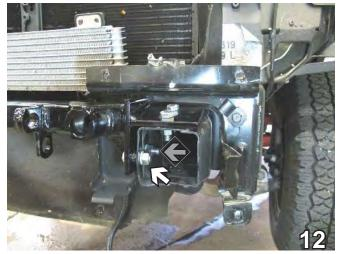
12. Hold spacer tube between the baseplate and frame rail and align to the front hole on baseplate side (see white arrow). In front hole of baseplate, insert the 1/2-13 x 1 1/2" bolt through spacer tube and tighten to the 1/2" lock washer and 1/2-13 hex nut on side of baseplate. In back hole, install bolt, lock washer and hex nut and tighten (see grey arrow). Do this to both sides of the vehicle.
