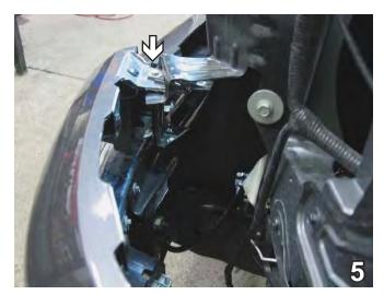
5. Using the 10mm socket, remove one metric bolt from the top of fascia. Do this to both sides of the vehicle. Set bolts aside to be reinstalled later.
