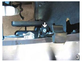
Behind front of fascia, on top of the frame, remove one metric bolt from the hood support bracket using the 10mm socket. Remove bracket. Do this to both sides of the vehicle. Set bolts and brackets aside to be reinstalled later.
