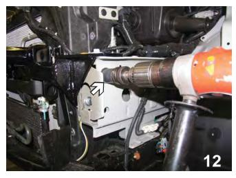
12. Using a 1 1/4" hole saw, drill two 1 1/4" holes into the frame, so an extension can be used to tighten up bolts. Do this to both sides of the vehicle.
