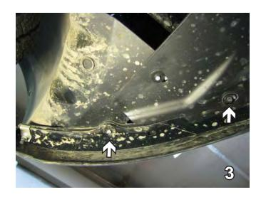
Using a 5.5MM socket, remove two bolts that are located underneath. Set bolts aside to be reinstalled later. Do this on both sides of the vehicle.
