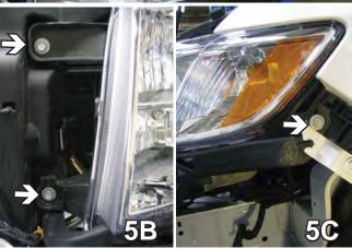
5. Using a 10MM socket, remove four bolts from the headlight assembly. Remove headlight by pulling it forward and disconnecting the electrical connections. Do this to both sides of the vehicle. Set headlight assemblies and bolts aside to be reinstalled later.
