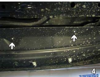
Using a flat screwdriver, remove three push pins across the middle. Set push pins aside to be reinstalled later. Pull the fascia up and out to remove from the vehicle and set aside carefully to be reinstalled later.
