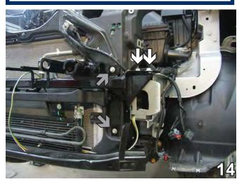
14. After the bolts in Step 13 are installed, you can reinstall the top two 13MM bolts (see white arrows) removed in Step 7 and also the two 10MM bolts (see grey arrows) removed in Step 7 to hold the radiator support back in place. Do this to both sides of the vehicle.
