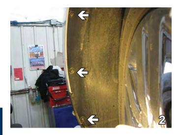
Using a 5.5MM socket, remove three bolts just forward of the front tire on the wheel well.
