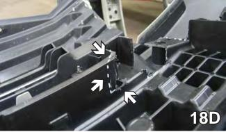
18. Using a reciprocating saw, trim away plastic areas located on the back side of the fascia, as indicated in photos 18A, 18B, 18C and 18D. Do this to both sides of the fascia.
