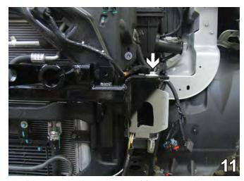
11. Place baseplate on top of frame and line up the holes in the baseplate with the existing holes on top of the frame. Insert one existing 13MM bolt removed in step 7, to hold baseplate into place. Do this to both sides of the vehicle. Use a floor jack to hold the radiator up in place.
