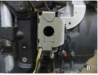
On the front of the frame, using a reciprocating saw, cut straight down on the dashed lines.
