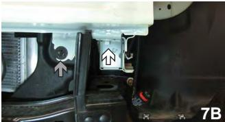
7. Using a 13MM socket, remove two bolts from the top of the metal bumper and one bolt from the bottom (see white arrows). Then using a 10MM socket, remove one bolt from the top of the bumper and one bolt from the bottom (see grey arrows). Do this to both sides of the vehicle. Set bolts aside to be reinstalled later and the metal bumper will not be reinstalled.
