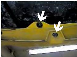
**5.** Remove the three metric bolts and three push pins the middle of fascia's lower edge, using the 10MM socket, pull fascia forward and set aside.
