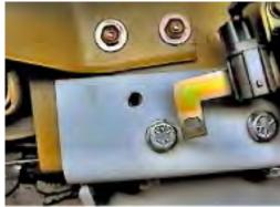
10. Align baseplate's upper front hole with existing front for solenoid on driver's side and clamp to frame with the vise grip. Note distance from frame end to baseplate front edge, apply same to the passenger's side and clamp to frame with vise grip.
