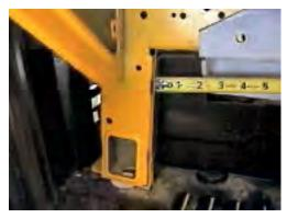
**8.** Measure 2" from the back edge of air dam forward, cut upper forward section with the utility knife, remove push pin and discard cut piece, both sides.
