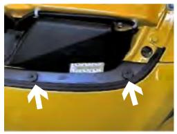
1. Remove the five phillips screws from black plastic cover on top side of fascia with the phillips screw driver, lift cover and set aside.
