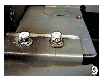
Using the 12MM socket, remove two metric bolts from the top of the metal bumper. Do this to both sides of the vehicle. Set the bolts aside to be reinstalled later. 10. Remove the metric bolt from the bottom of the metal bumper with the 12MM socket. Pull the metal bumper forward to remove. The metal bumper will not be reinstalled.
