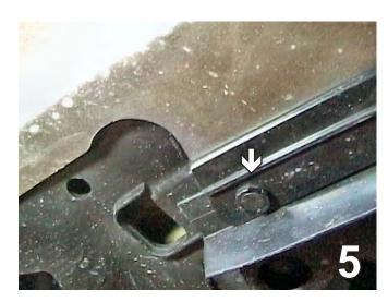
Remove the six pushpins from the lower edge of the fascia and the belly pan. Pull the fascia forward to remove. Set the pushpins and fascia aside carefully to be reinstalled later.
