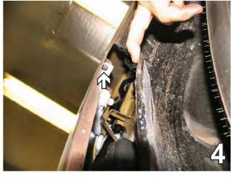
Using the Phillips screwdriver, remove the Phillips screw from the corner of the fascia just forward of the front tire, inside the wheel well cover. Do this to both sides of the vehicle.
