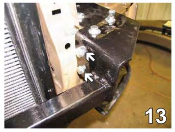
13. Using the baseplate as a template, drill the two holes in the side of the baseplate into the frame with the 13/32" drill bit. Do this to both sides of the vehicle. Insert the nutplate into the end of the frame to align with the drilled holes, tighten the 3/8" x 1 1/2" hex bolt and lock washer with the 9/16" socket. Do this to both sides of the vehicle. (**LOCTITE**)
