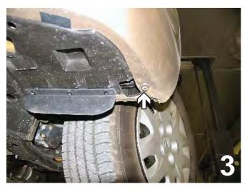
3. Using a 10MM socket remove one metric bolt from just forward of the front tire. Do this to both sides of the vehicle.
