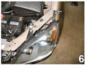
6. Remove one metric bolt, as indicated by the white arrow in the photo above, with the 10MM socket and one pushpin, as indicated by the grey arrow in the photo above, from the top side of the headlight assembly. Do this to both sides of the vehicle. Set the bolts and pushpins aside to be reinstalled later.
