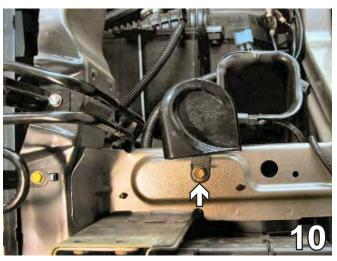
10. On the frame support, just forward of the air intake, use a 12mm socket to remove the bolt securing the horn bracket. Move the horn and bolt out of the way to open up this area for drilling. Do this to both sides of the vehicle.
