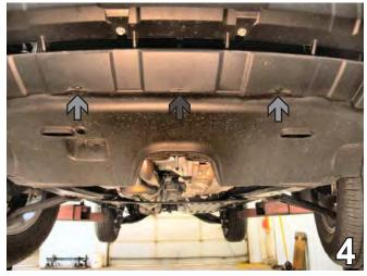
4. Below the fascia-wide horizontal opening on the bottom of the fascia, remove three pushpins (see grey arrows in photo above). Pull upper corners of fascia outward, to the side of the vehicle, releasing three clips. Pull fascia forward, releasing it from clips under the headlight. Do this to both sides of the vehicle. Pull fascia forward to remove. Set pushpins, bolts, and fascia carefully aside to reinstall later.
