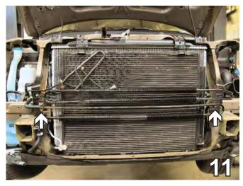
11. Using a 10mm socket, remove the two metric bolts securing the coolant line to either side of the radiator support. Set bolts aside to reinstall later.
