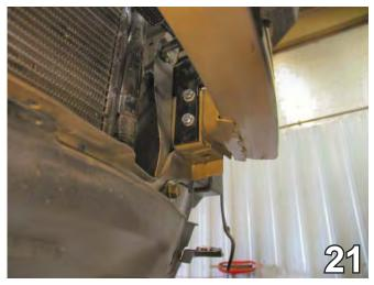
21. With the bumper off, insert 3/8-16 nutplate into the frame opening to align with drilled holes on the side of the frame rail. Insert the two 3/8-16 x 1 1/2" hex bolts and 3/8" lock washers and hand tighten. Metal bumper is only shown in photo for orientation
