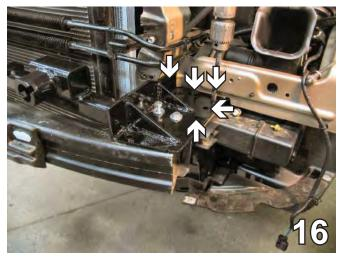
16. Using the baseplate as a template on the drivers side, begin drilling holes using the 13/32" drill bit. Do not insert any bolts at this time. Drill four holes into the frame rail, one into the radiator support, and one into the bumper from the top of the baseplate. Do this to both sides of the vehicle.
