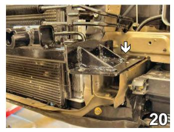
20. Slide the baseplate onto the frame rail and align with the holes in the frame rail. With the bumper off, insert 3/8-16 nut plate into the frame opening to align with the drilled hole in the rear of the baseplate (closest to radiator support). Insert a 3/8-16 x 1 ½ hex bolt and 3/8" lock washer and hand tighten to the nut plate. Do this to both sides of the vehicle.
