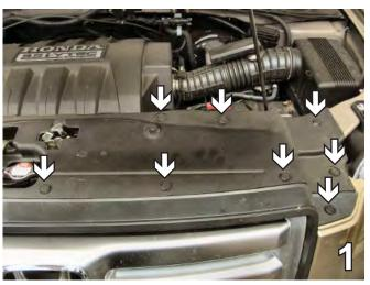
1. Remove 15 pushpins from the plastic on top of the fascia. Set plastic and pushpins aside to reinstall later. The driver's side is shown in photo above.
