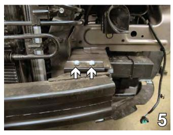
5. Release the temperature sensor from its clip (not shown) found behind the metal bumper and set aside to reinstall later. Using a 12mm socket, remove two metric bolts from the top of the metal bumper. Do this to both sides of the vehicle. Set bolts aside to be reinstalled later.
