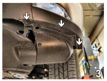
On the bottom edge of fascia, remove a pushpin and two metric bolts using a 10MM socket. Do this to both sides of the vehicle. Set pushpins and bolts aside to reinstall later.
