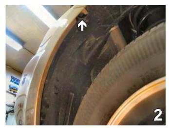
Above the front tire, inside the wheel well on the edge of the fascia, remove one Phillips screw. Do this to both sides of the vehicle. Set screws aside to reinstall later.
