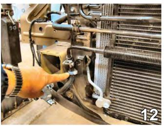
12. On the passenger's side, release the hose clamp found near the frame rail and slide the hose out of the clamp. Swivel the coolant line and hose to the left of the radiator support – moving the coolant line and hose away from the frame rail to clear that area for drilling.
