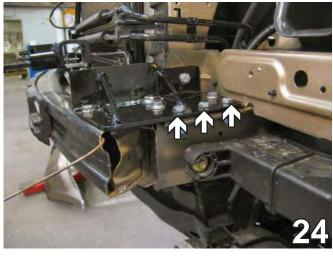
24. Insert three 3/8-16 x 1 ¼ hex bolts into the baseplate holes that and align the backing plate with bolts. Tighten with 3/8" flat washers, 3/8" lock washers, and 3/8-16 hex nuts. Do this to both sides of the vehicle.
