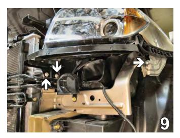
9. Using a 10mm socket, remove two metric bolts at the bottom of the headlight assembly near the radiator support (see square in photo above). On the bottom edge of headlight assembly, just below front fender, use a 10mm socket to remove one metric bolt. In the same area, remove one pushpin. Pull headlight assembly forward and disconnect electrical connections. Set bolts and headlight assembly aside to reinstall later. Do this to both sides of the vehicle.
