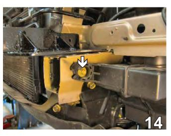
14. On the driver's side, using a 10mm socket, loosen the metric bolt securing the air intake baffle to the frame rail. Move the baffle down and out of the way to clear an area for drilling.
