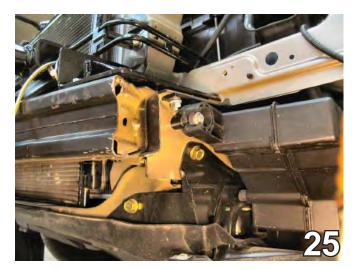
25. Move the air intake baffle back to its original position. Using a 10mm socket, secure to the frame rail with a 3/8 spacer tube and 6mm-1 x 50 hex bolt.
