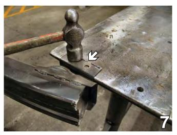
7. Lay the metal bumper's upper bracket on a solid metal surface. Pound the ridge on the bracket to flatten it and prepare it for baseplate installation. Do this to both sides of the metal bumper. Set bumper aside to reinstall later.
