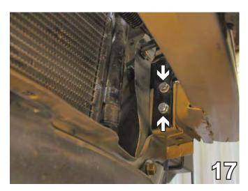
17. On the driver's side, on the side of the frame rail facing inward toward the radiator, use the 13/32" drill bit to drill two holes using the baseplate as a template. Do this to both sides of the vehicle. Do not insert any bolts yet. Bolts are only shown in photo for orientation.
