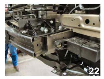
22. Slide the metal bumper between baseplate and the frame to align baseplate, metal bumper and existing bolt locations for the metal bumper. Insert and tighten the two 8MM bolts, 3/8" lock washers, and 3/8" flat washers. Do this to both sides of the vehicle. **TIGHTEN ALL REMAINING BOLTS.**
