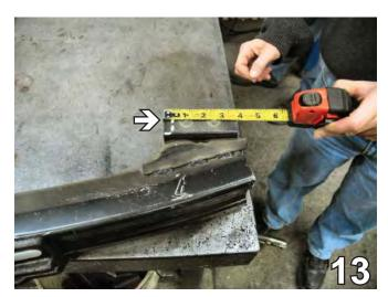
13. Mark and cut a section of the top bumper bracket edge that faces toward the center of bumper. Using the reciprocating saw, make a horizontal cut on the top of the bracket removing 3/8" from the end of the bracket. Do this to both sides of the bumper.
