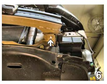
Using a 12mm socket, remove one metric bolt from the bottom of the metal bumper. Do this to both sides of the vehicle. Pull the bumper forward to remove. Set bolts and metal bumper aside to be reinstalled later.
