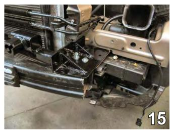
15. Slide the baseplate onto the top of the frame rail and guide the metal bumper between baseplate and the top of the frame rail. Align the two holes of the baseplate with the two holes on top of the metal bumper and frame. Insert two 8mm-1.25 x 30mm hex bolts and fasten (do not overtighten) with 8mm lock washer and 5/16" flat washer using a 13mm socket. Do **NOT** use Loctite yet.
