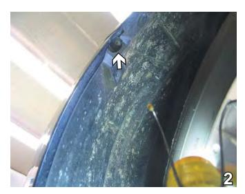
Just inside wheel well, on edge of fascia, remove one Phillips screw. Do this to both sides of the vehicle. Set screws aside to be reinstalled later.
