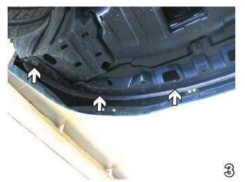
Remove eight pushpins from bottom of fascia (three each side and two in the center). Pull upper corners of fascia to the side to release tabs. Do this to both sides of the vehicle. Pull fascia forward to remove. Set pushpins and fascia aside to be reinstalled later.
