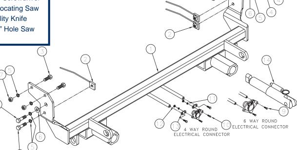
Use only genuine factory replacement parts on your baseplate. Do **NOT** substitute homemade or non-typical parts. If a bolt is lost or in need of replacement, for your safety and the preservation of your baseplate, be sure to use a replacement bolt of the same grade (In most cases it will be Grade 5, please reference the parts list above). Replacement parts may be ordered through your nearest Blue Ox® Dealer or Distributor.
