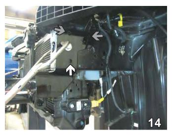
14. On the driver's side, use the baseplate as a template and drill the three remaining holes using the 13/32" drill bit. Insert 3/8" nut plate through frame end hole and align to the bottom hole (see white arrow). Install 3/8-16 x 1 ½" hex bolt with 3/8" lock washer and tighten to nut plate. On upper two holes, install 3/8-16 x 1" hex bolt from the backside of the upper frame webbing and tighten to the 3/8" lock washers and 3/8-16 hex nuts on the outside of baseplate (see grey arrows).
