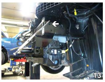
13. On the driver's side, use the baseplate as a template to drill the front center hole in the frame with the 13/32" drill bit. Insert 3/8" nut plate through frame end hole and align to the drilled hole. Install 3/8-16 x 1 ½" hex bolt with 3/8" lock washer and 3/8" flat washer and tighten to nut plate.
