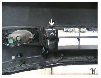
11. On the driver's side, mark the upper air vent flush with the back side of the grille opening. Using the utility knife, trim the marked area.
