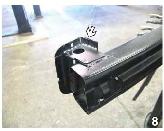
8. With the bottom of the metal bumper face up, mark the back of bumper bracket webbing so it is flush with the bottom edge of bumper. Using the reciprocating saw, cut the marked area to remove lower webbing. Do this to both sides of the vehicle.
