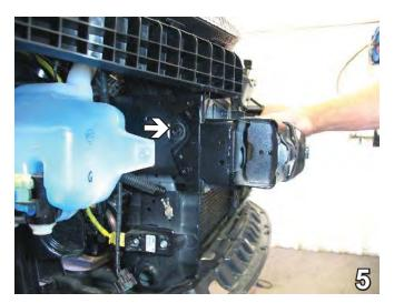
On the passengers side, remove one metric bolt from the side of the metal bumper using the 12mm socket. Set bolt aside to be reinstalled later.
