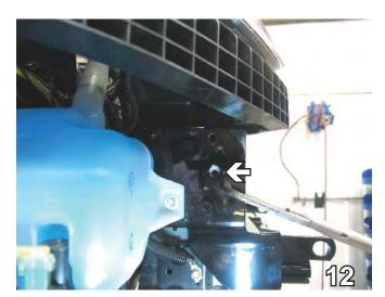
12. Align the baseplate with passenger's side existing hole, top and front edge of the frame rail. Clamp in place using the vice grips. Install the 8mm hex bolt with 3/8" lock washer and 3/8" flat washer to the existing hole and tighten. Using the baseplate as a template, drill the three remaining holes in the passenger's side frame with the 13/32" drill bit.
