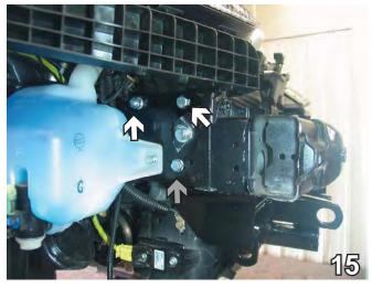
15. On the passenger's side upper two holes, install 3/8-16 x 1" hex bolts from the upper frame webbing and tighten to the 3/8" lock washers and 3/8-16 hex nuts on the outside of baseplate (see white arrows). Insert 3/8" nut plate through frame end hole and align to the bottom hole (see grey arrow). Install 3/8-16 x 1 ½" hex bolt with 3/8" lock washer and tighten to nut plate.
