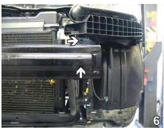
Using the 12mm socket, remove two metric bolts from the metal bumper. Do this to both sides of the vehicle. Pull metal bumper forward to remove. Set bolts and metal bumper aside to be reinstalled later.
