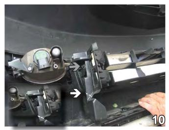
10. Lay fascia face down on a smooth, flat surface. Using the utility knife, trim horizontally across the fascia support molding next to the grille (see white arrow). Remove one Phillips screw from the fascia support (see grey arrow). Remove upper portion of fascia support. Do this to both sides of the vehicle.
