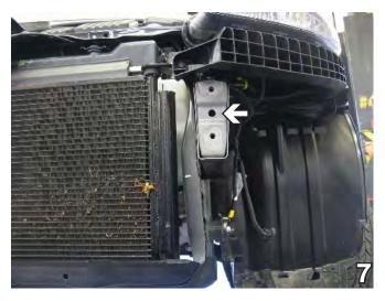
7. Using the 1 1/4" hole saw, ream out the center hole on the end of the frame rail. Do this to both sides of the vehicle.
