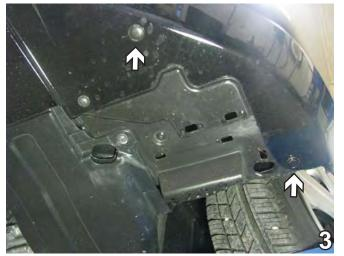
3. Remove two pushpins from bottom of fascia in the corner. Set pushpins aside to be reinstalled later.
