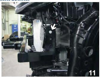
Align the baseplate with the drilled out hole. Be sure the baseplate is level. Fasten on with a 1 1/4" bolt and 3/8" hex nut. Use the baseplate as a template to drill the other two holes. Do this on both sides.
