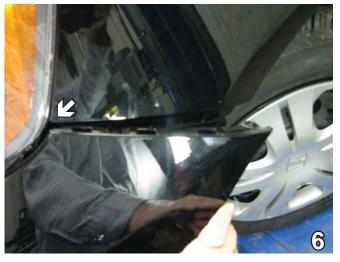
6. Grab the strip under the headlight and pop out all along under the headlight. Do this to both sides of the vehicle. Pull upper corners of fascia to the side. Do this to both sides of the vehicle. Pull fascia forward to remove. Set strip and fascia aside to be reinstalled later.
