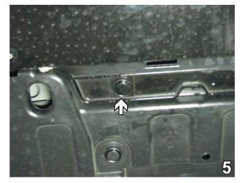
5. Remove three pushpins from across the edge. Set pushpins aside to be reinstalled later.
