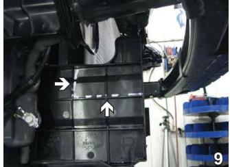
9. On the passenger side, also trim the plastic using a utility knife.
