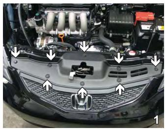
1. On top of the fascia, remove eight pushpins. Set pushpins aside to be reinstalled later.
