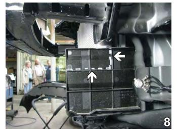
8. Using the utility knife, cut the plastic on the driver's side as shown.
