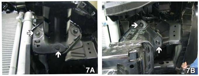
7. Using the 12mm socket, remove four bolts from the metal bumper. Do this to both sides of the vehicle. Pull metal bumper forward to remove. Set bolts and metal bumper aside to be reinstalled later.
