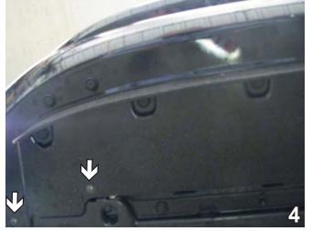
4. Using a Phillips screwdriver, remove two screws from under the fascia. Set screws aside to be reinstalled later.
