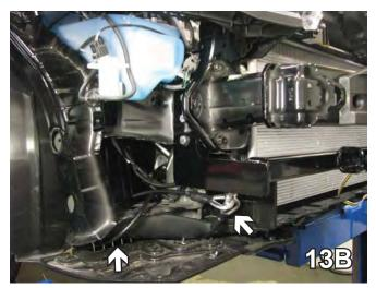
13. Attach the permanent baseplate safety cables to the provided convenience link on the baseplate. Secure the cable to a solid piece of the vehicle's frame as described in the instructions included with the permanent baseplate safety cables. 14. After the baseplate has been installed. Reinstall metal bumper, strip, fascia, pushpins, bolts and screws.
