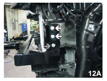
12. In the top two holes, insert 1 1/4" bolts (12A white arrows). On the inside of the frame end, attach to a plate with the narrow end to the front with 3/8" lock nuts (12B). In the bottom hole, insert 1 1/2" bolts (12A gray arrow) and attach to 3/8" lock nuts underneath on the webbing (12C). Use Loctite Red on all bolts. Do this on both sides.
