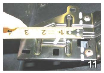
11. Cut the fog light bracket on the white line. Replace the housing to the bracket and reattach back to the fascia. Do this on both sides.
