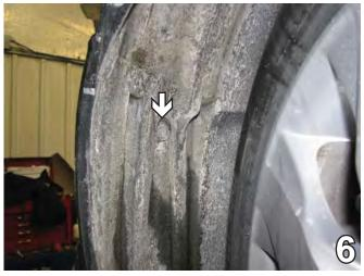
6. On the driver's side, remove the push pin just forward of the front tire in the wheel well. Set the push pin aside to be reinstalled later.
