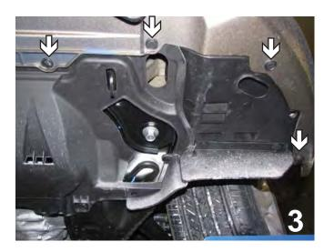
Underneath the fascia, remove ten push pins all the way around. Set push pins aside to be reinstalled later.
