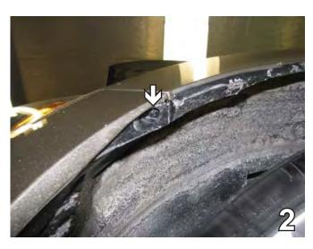
2. In the corner of the fascia, remove the Phillips screw. Do this to both sides of the vehicle. Set screw aside to be reinstalled later.
