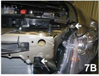
7. Remove the headlight by removing the three bolts around it and unplug the electrical connections. Do this on both sides. Set the bolts and headlights aside to be reinstalled later.
