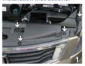
Remove eight push pins in order to remove the radiator cover. Do this to both sides of the vehicle. Set cover and push pins aside to be reinstalled later.
