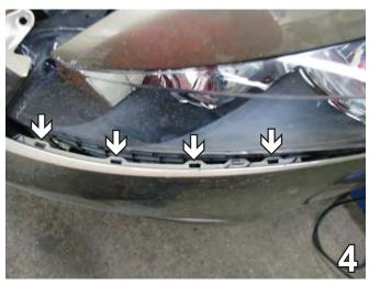
4. Pull the fascia out up to the blinker. Use a small flat screw driver to pry down on each clip in the series of four in order to release the fascia. Pull the two eyelets up off the pins. Do this on both sides. Slide the fascia off, disconnect fog lights and set aside carefully to be reinstalled later.
