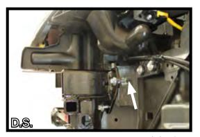
17. Insert one (1) 1/2"-13 x 1-1/2" bolt and 1/2" lock washer into the side hole. Use one (1) of the 1/2"-13 nut plates to fasten securely.
