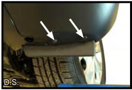
3. Remove the one (1) screw and one (1) push pin that are on the under side of the vehicle, right ahead of the front tire.
