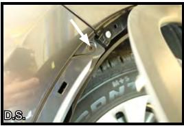
5. Carefully pry the wheel well trim back slightly. With a Phillips screwdriver remove the one (1) screw that is located towards the top portion of the wheel well.
