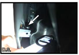
2. Gently pull the wheel well liner back. Remove the push pin that is located along the lower, outside edge.
