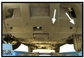
4. Remove the four (4) push pins that are located under the vehicle. There are two (2) on the passenger's side and two (2) on the driver's side.
