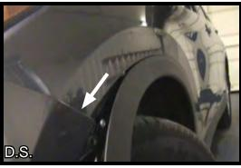
6. Pull the front fascia up and outward to remove. Apply slight pressure as this does not pull away easily.
