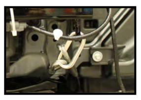
23. Attach the permanent baseplate safety cables to the provided convenience link on the baseplate. Additional options may interfere with suggested mounting; in this case, secure the cables to a solid piece of the frame as described in the instructions included with the permanent baseplate safety cables. Be sure the safety cables do not rub against any hoses and/or moving parts. Do this on both sides of the vehicle.
