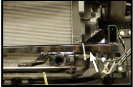
20. Using the cable tie that was provided, relocate the temperature sensor by attaching it to the baseplate.
