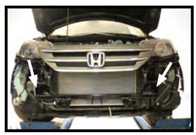
15. Slide the tubes of the baseplate assembly into the rectangular tube on the vehicle frame.
