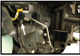
19. Make sure the coolant line does not interfere with the attachment tab. Snap coolant line back into bracket.
