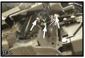
16. Align the bolt holes. Insert the three (3) 8MM-1.25 x 30MM bolts, 8MM lock washers and 8MM flat washers. Do not tighten at this time. Once all the fasteners have been started and the plate is properly aligned tighten all fasteners securely.
