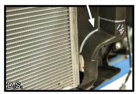
12. Additional cutting is required on the rubber mounts located next to the radiator. Mark each per image above and notch accordingly.
