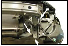
8. Using a 12MM socket, remove the four (4) bolts on the bumper core. There is one (1) on the top, one (1) on each side and one (1) on the bottom. Do this on both the sides of the vehicle.
