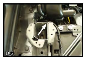
13. Using a chisel, remove the nut in order to slide the baseplate in.
