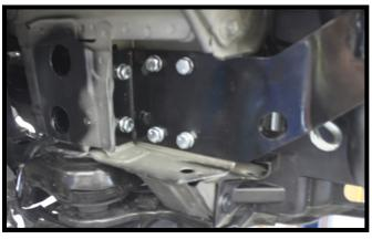
10. Continue to drill the remaining holes thru the frame. Install 3/8"-16 x 1-1/2" bolts with a 3/8" lock washers into the holes and secure with a 3/8" nut plates on the inside of the frame. Do this on both sides of the vehicle. Fully tighten all fasteners.
