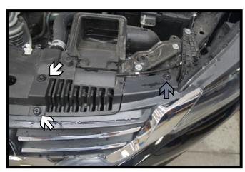
Remove the four (4) push pins from the fascia cover (white). There are two (2) on each side and set aside. Remove the two (2) push pins from the outer edges of the top of the fascia (gray). There is one (1) on each side.
