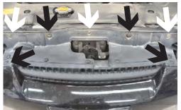
1. Remove the four push pins (black arrows) and three phillips screws (white arrows) along the back edge of black plastic cover on top side of fascia with the phillips screw driver. Llft cover and set aside.
