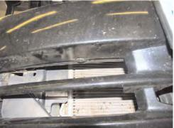
7. Remove one phillips push pin from the underside of grill opening with the phillips screw driver, both sides, pull fascia forward and carefully set aside.
