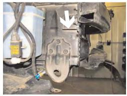
8. Remove the three metric bolts from tie down bracket with the 17MM socket, both sides. Using the reciprocating saw, cut support rib on the side of frame just behind frame end and bend rib down flat against frame with a hammer, both sides.
