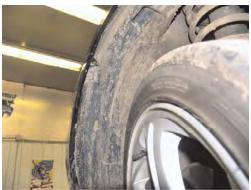
2. Remove two metric bolts just forward of front tire on corner of fascia and edge of wheel well with the 8MM and 10MM socket, both sides.
