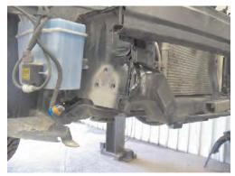
**10.** Spray paint the cut edges of ribbing on both sides with a fast drying spray paint to prevent corrosion.
