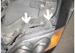
4. Remove two metric bolts from the top side of head light assembly with the 10MM socket, both sides.
