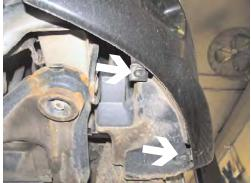
3. Remove two phillips push pins from lower edge of fascia just forward of front tires, both sides.
