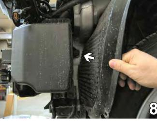
8. Remove the metric bolt from between the air baffle and wheel well using the 12MM socket, pull the air baffle down to disconnect from upper tube and set
