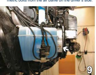
Remove front metric bolt from the washer reservoir on the passenger's side using the 10MM socket. Remove one Phillips screw, pull reservoir down, unplug electrical connections, disconnect and plug water lines, set aside.
