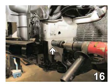
16. Using the 1 1/4" hole saw, cut an opening in the lower portion of the frame rail to use for wire nut installation, both sides as shown in photo.
