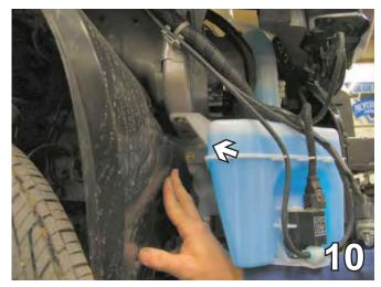
10. Separate the wheel well from the back side of the reservoir and remove the two metric bolts using the 10MM socket, pull reservoir down, unplug electrical connections, disconnect and plug water lines, set aside.
