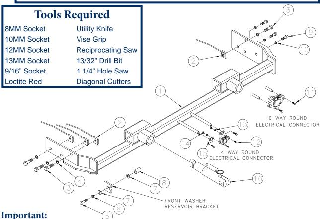
Use only genuine factory replacement parts on your baseplate. Do NOT substitute homemade or non-typical parts. If a bolt is lost or in need of replacement, for your safety and the preservation of your baseplate, be sure to use a replacement bolt of the same grade. In most cases it will be Grade 5-please reference the parts list above. Replacement parts may be ordered through your nearest Blue Ox\* dealer or distributor, or call our Customer Care Team at (402)385-3051 or toll free (888) 425-5382.
