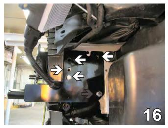
16. On driver's side, insert the 3/8-16 x 1 1/2" hex bolts and 3/8" lock washers into front and upper and lower holes and upper back hole, as indicated by the white arrows in the photo. Insert 3/8-16 x 1" hex bolt and 3/8" lock washer, 3/8" flat washer and 3/8" hex nut into the lower back hole, as shown by the grey arrow in the photo above. Tighten the lower bolt according to the torque specs on the front of these instructions or on page 3 of the Baseplate Towing General Instructions.
