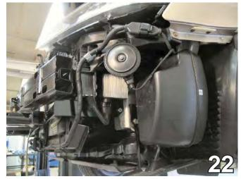
22. Reinstall horn to its original location. Be sure all electrical connections are plugged in properly.
