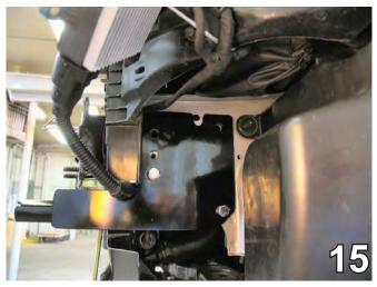
15. Using the baseplate as a template, drill five holes in the baseplate endplate with the 13/32" drill bit. Do this to both sides of the vehicle, the driver's side is shown.
