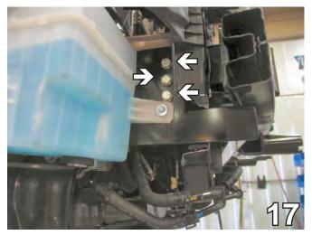
17. On passenger's side insert 3/8-16 x 1 1/2" hex bolt and 3/8" lock washer into 3 front holes, as indicated by the arrows in the photo above and upper back hole. Insert 3/8-16 x 1" hex bolt and 3/8" lock washer, 3/8" flat washer and 3/8" hex nut into lower back hole, located behind the washer reservoir in this photo.
