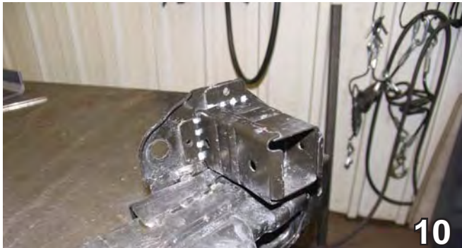
10. Using a reciprocating saw, cut bumper horn off flush with the base. Please refer to the photo above for reference. Do this to both sides of the metal bumper.
