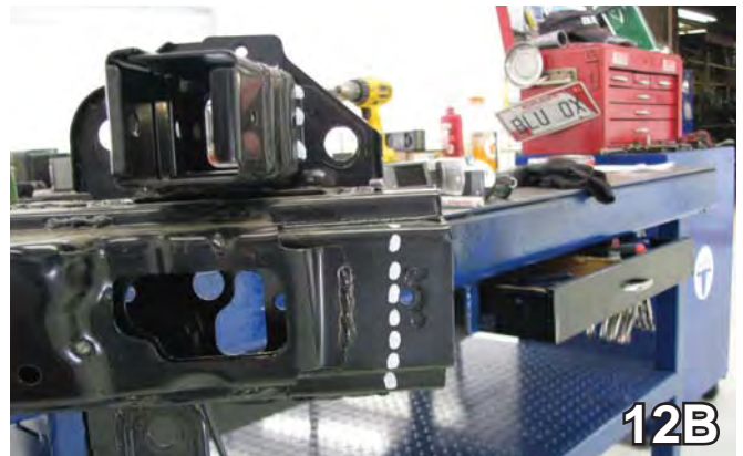
12. Using a reciprocating saw, cut off the end of the metal bumper. Do this to both sides of the vehicle.
