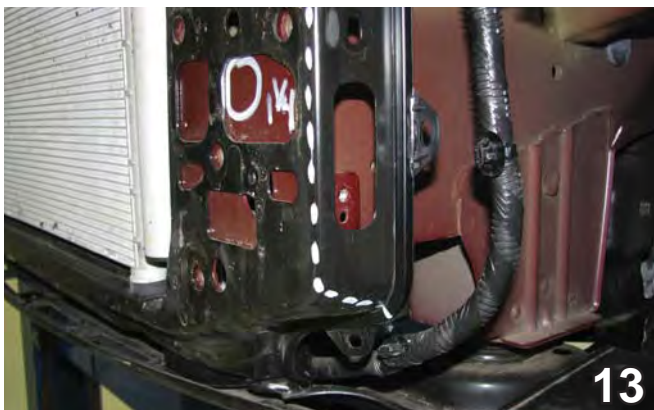
13. Using a 1 1/4" hole saw, drill a hole into the frame as shown. This needs to be done so that the top two bolts of the metal bumper can be reinstalled after the spacer plates are put on. Do this to both sides of the vehicle.
