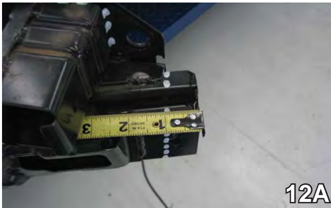
12. Using a reciprocating saw, cut off the end of the metal bumper. Do this to both sides of the vehicle.
