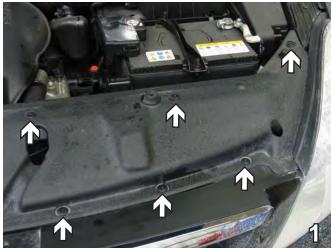
Using a Phillips screwdriver, remove thirteen plastic Phillips push pins all together from the top plastic piece. There are six push pins located on the driver side and passenger side and one push pin in the middle. Set push pins aside to be reinstalled later.
