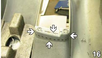
16. Using a reciprocating saw, trim next to the bolt holes and down about 5/8". Reinstall headlights, fascia, bumper, bolts and push pins.
