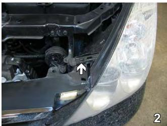
Using a 10MM socket, remove one metric bolt located by headlight. Do this to both sides of the vehicle. Set bolts aside to be reinstalled later.
