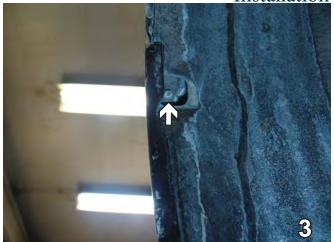
Use a 8MM socket for the Hyundai, a 10MM for the Kia, remove one metric bolt just forward of the front tire, on the wheel well. Do this to both sides of the vehicle. Set bolts aside to be reinstalled later.
