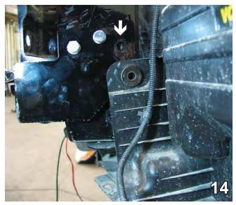
14. Remove existing bolt from baseplate and bolt the air dam back into place. Before you reinsert the bolt, place a flat washer on and then tighten down.
