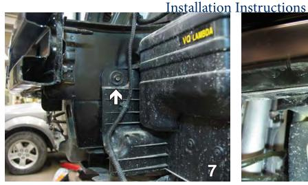
Using a 10MM socket, remove one metric bolt located near the air dam on the driver side of the vehicle. Set bolt aside to be reinstalled later.
