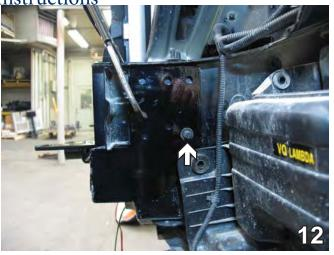
12. On driver side, insert bolt removed in Step 7 and tighten down. This is just to hold baseplate in place so the other holes in the baseplate can be drilled. The bolt will be removed again so the air dam can be put back into place.
