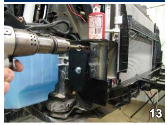
13. Using the baseplate as a template, drill the remaining holes into the frame with a 13/32" drill bit. Insert the nut plates into the frame and align with drilled holes. Insert a 3/8-16x1 1/4" hex bolt and 3/8" lock washer into the holes and tighten down with nut plates.
