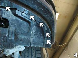
4. Using a Phillips screwdriver, remove thirteen plastic Phillips push pins located just forward of the front tire along the bottom edge of fascia, from the driver side to the passenger side of the vehicle. Set push pins aside to be reinstalled later.
