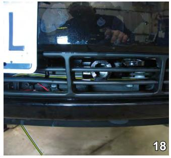
18. Align the fascia to its original position and using a hack saw blade, remove area around attachment tab receiver to allow for it to come through the fascia. Do this to both sides of the vehicle.
