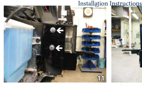
11. Slide baseplate up so that the holes on the baseplate line up with the existing holes in the frame on the passenger side. Clamp baseplate in place with vise grips. Insert a 8MM-1.25x30MM hex bolt, 3/8" lock washer and 3/8" flat washer into the two existing holes and tighten down.
