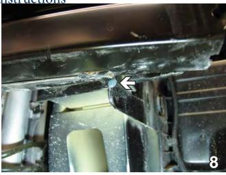
8. You will need to grind off a small tab, indicated in the photo above on the driver side only.
