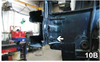
10. Using a 12MM socket, remove two bolts located on top of the metal bumper and a nut located on the back side of the metal bumper. Do this to both sides of the vehicle. Set metal bumper, bolts and nuts aside to be reinstalled later.
