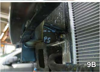
You will need to trim the plastic piece located under the metal bumper so it's flush with the bottom of the bumper. Do this to both sides of the vehicle.
