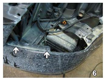
6. Once headlight assembly is removed, you will need to remove one metric bolt with a 10MM socket and two plastic Phillips push pins with a Phillips screwdriver. Do this to both sides of the vehicle. Set bolts and push pins aside to be reinstalled later. The fascia is then ready to be removed from the vehicle and set aside carefully to be reinstalled later.
