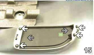
15. Remove the covering (grey arrows) from inside the bumper. Using a 7MM socket, remove four bolts. Do this on both sides. The bolts will be reinstalled after trimming.
