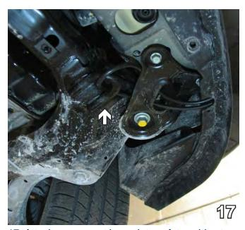
17. Attach permanent baseplate safety cables to the convenience link on the baseplate. The photo above shows recommended installation of the cables to frame of vehicle. If vehicle has additional options (not shown above) which interfere with mounting permanent baseplate safety cables, secure the cables to a solid piece of the vehicle frame as described in instructions included with the permanent baseplate safety cables.
