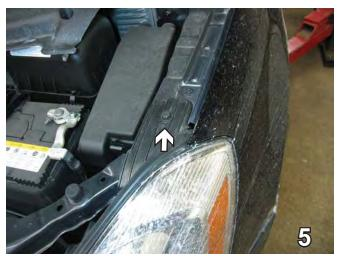
5. On the Hyundai, using a 10MM socket, remove bolt from headlight assembly and then pull headlight forward to remove. Do this to both sides of the vehicle. Set headlight assemblies and bolts aside to be reinstalled later.
