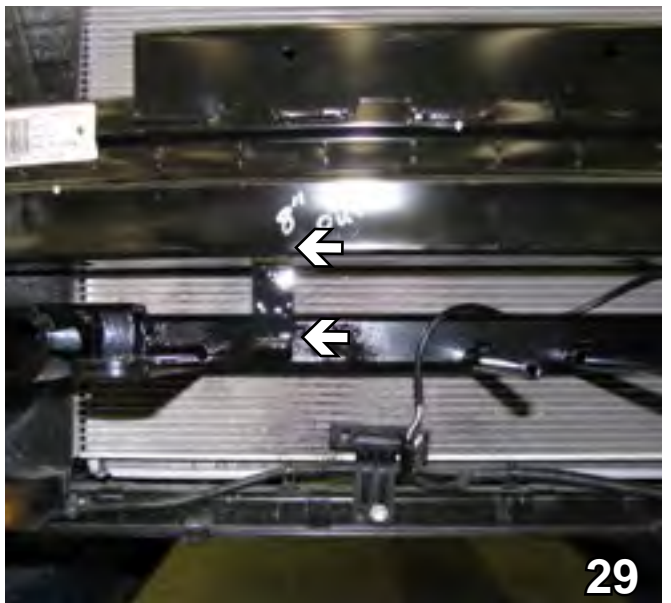
29. Using a 13/32" drill bit, drill through the existing hole in the bottom of the bumper. Attach the breakaway bracket with a 1/4-20 x 2 1/2" hex bolt and 1/4-20 hex nut. Attach the breakaway to the bracket with 1/4-20 x 3/4" hex bolt and 1/4-20 hex nut.
