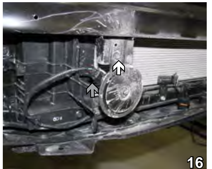
16. Using the 10MM socket, remove the bolt attaching the horn to the bracket (white arrow). Unplug the horn (gray arrow). Set the horn and the bolt aside to be reinstalled later.
