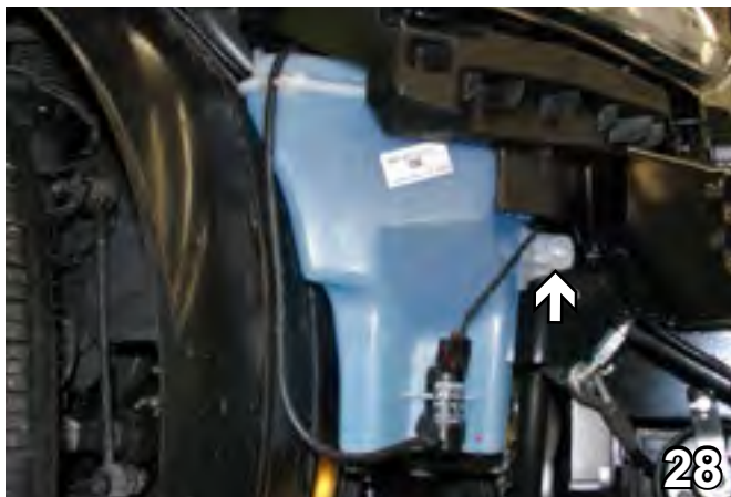
28. Reinstall the washer reservoir with a 6MM-1 x 30MM hex bolt, 1/4" lock washer and 1/4" flat washer into the existing hole on the baseplate. Use the existing bolts previously removed to tighten the other side. Reconnect the hoses.
