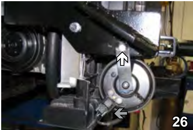
26. On the passenger side, mount the horn on the bottom hole with a 1/4-20 x 3/4" hex bolt to a 1/4-20 hex nut (white arrow) . Reconnect the plug (gray arrow).
