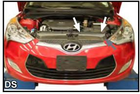
1. With a 10mm socket, remove the two (2) bolts on the top portion of the fascia. Using a flat screwdriver, release the push pin.
