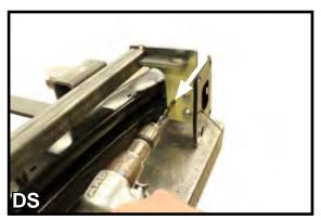
11. Using the baseplate end plates as a guide, drill an additional 13/32" hole on both sides.
