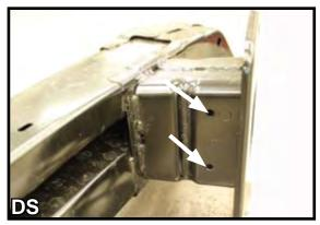
9. Ream out the existing two (2) holes on both side of the bumper using a 13/32" drill bit.
