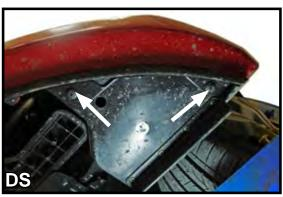
2. With a phillips screwdriver, remove the two (2) screws from the underside of the fascia.
