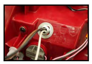
2. Drill a 1" hole to install the 3 wire automotive socket.
