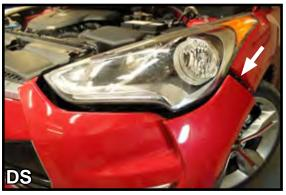
4. Pull the side of the fascia slightly downward away from the headlights. Lift the side upward and gently away from the vehicle. Place the front fascia to the side during baseplate installation.
