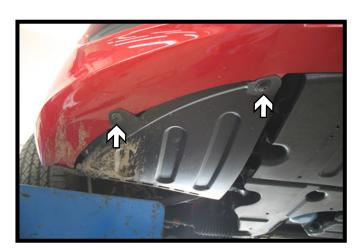
Remove the four (4) Phillips head push pins from the underside of the fascia. There are two (2) on each side.
