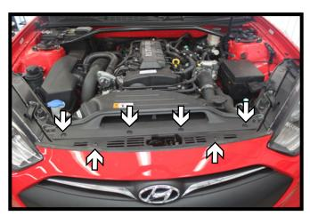
1. Remove the six (6) Phillips head push pins from the top edge of the fascia.
