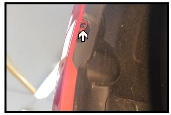
Using a 8MM socket or Phillips screwdriver, remove the screw from the top edge of the wheel well. Do this on both sides of the vehicle.
