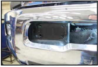
Using a 16MM socket, remove the four (4) bolts from the tow hook and remove from the vehicle. DO NOT discard the factory nuts they will be reused to install the baseplate. Repeat on the other side of the vehicle.
