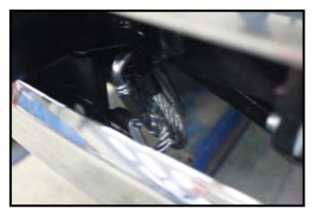
3. Attach the permanent baseplate safety cables to the provided convenience link on the baseplate. The photo above shows the recommended installation of the cables to frame of vehicle. Additional options may interfere with suggested mounting; in this case, secure the cables to a solid piece of the frame as described in the instructions included with the permanent baseplate safety cables. Be sure the safety cables do not rub against any hoses or moving parts. Do this on BOTH sides of the vehicle.
