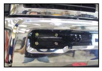
Using a 16MM socket/wrench, install the baseplate and tow hook into the tow hook holes using the 10MM-1.5 x 50MM bolts, 10MM flat washers and existing nuts. Repeat on the other side of the vehicle.
