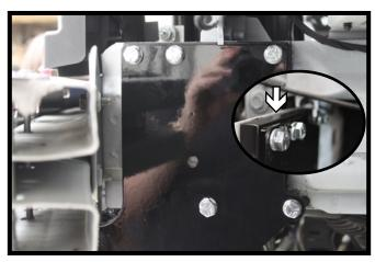
16. Using a 13/32" drill bit, drill the top three (3) holes and bottom two (2) holes into the frame. Install a 3/8"-16 x 1-3/4" bolt, 3/8" lock washer and 3/8"-16 nut into the each of the holes. On the top holes use the spacer plate between the frame and baseplate. Tighten down all fasteners. Do this on both sides of the vehicle.
