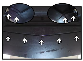
Using a 7MM socket, remove the nine (9) screws from the bottom edge of the fascia.
