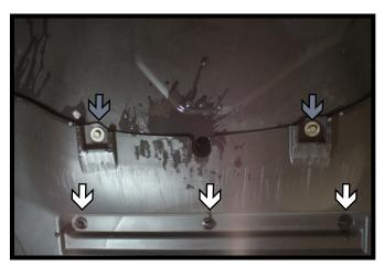
10. On the underside of the vehicle remove the plastic sheilding. Remove the three(3) push pins (white). Then using a 10MM socket, remove the two (2) bolts (gray).
