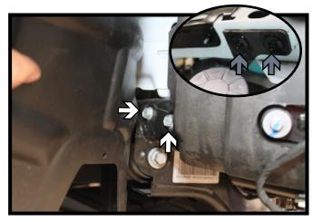
11. On the passenger side the power steering pump will need to be dropped down for clearance. Using a 10MM socket, remove the two (2) bolts from the rear bracket (white) and the two (2) bumper bracket bolts (gray).
