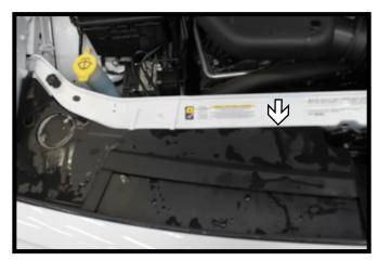
Lift up and remove the plastic radiator covers from both the passenger and driver side of the vehicle.
