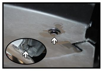
9. Remove the plastic shrouding on the driver side. On the top side, remove the rear push pin and the upper push pin (left). On the underside of the shrouding, remove the bottom push pin and the push pin located just inside the wheel well (right)
