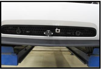
21. Hold the fascia as close to it's original position, mark and trim the lower grille as needed for baseplate clearance. Reinstall the plastic fascia support, fascia and underside shielding.
