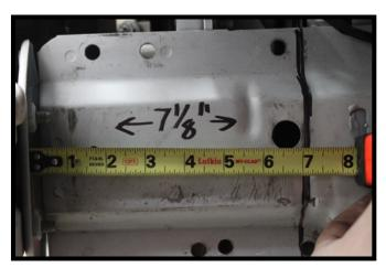
14. Measure back from the backside of the frame end plate 7-1/8" and make a mark. Do this on both sides of the vehicle.
