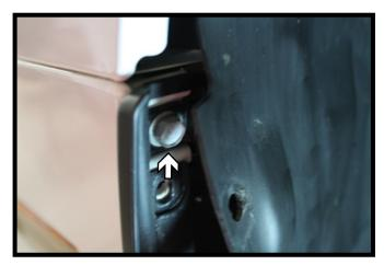
4. Using a 10MM socket, remove the screw from behind the wheel well cover at the top edge of the fascia. Do this on both sides of the vehicle.
