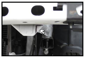
13. Using a reciprocating saw, notch the frame end flush with the bottom of the bumper and flush with the outside of the frame. Do this on both sides of the vehicle.
