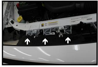
Remove the six (6) push pins from the top side of the fascia. Three (3) push pins from both sides of the vehicle.
