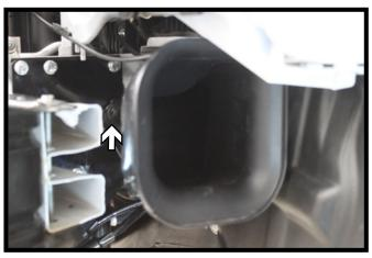
18. Reinstall the air baffle, using the existing hole thru the baseplate.
