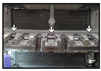
7. Remove the three (3) push pins from the plastic fascia support and unsnap from the metal bumper.
