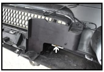
20. Before reinstalling the fascia, remove the plastic sheilding from both sides by removing the plastic rivets.
