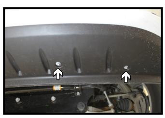
1. Using a 10MM socket, remove the four (4) screws from the front spoiler. There are two (2) on each side.
