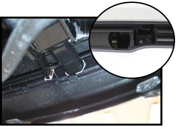
Temporarily reinstall the front cover. Hold the baseplate up as close to its installed position. Mark the backside of the front cover. Remove and trim the cover to allow the baseplate to pass thru. Do this on both sides of the vehicle.
