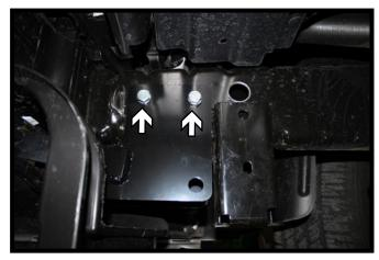
Using a 17/32" drill bit, drill the upper two
