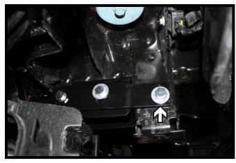
10. Using a 17/32" drill bit, drill the rear side plate hole thru the tow hook bracket. Install a 1/2"-13 x 1-1/2" bolt with 1/2" lock and flat washers into the hole with 1/2" nut wires on the inside of the bracket and tighten. Do this on both sides of the vehicle.
