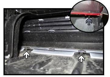
Remove the seven (7) push pins (white) and the two (2) plastic rivets (gray) from the inside edge of the spoiler where it meets the bumper. Set the spoiler aside.
