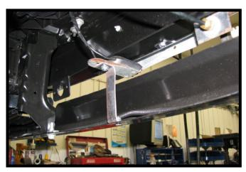
13. The breakaway bracket can be attached to the bottom edge of the bumper using a 1/4"-20 x 3/4" bolt with a 1/4"-20 nut. Trim the front cover (not shown) as needed to allow the breakaway to pass thru and attach the breakaway to the top of the bracket with a 1/4"-20 x 3/4" bolt and a 1/4"-20 nut.
