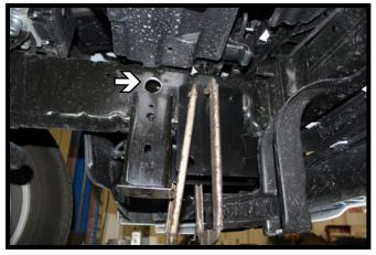
Clamp the baseplate into position. Using a 1-1/4" hole saw, drill an access hole above the tow hook bracket on the inside of the frame. Do this on both sides of the vehicle.
