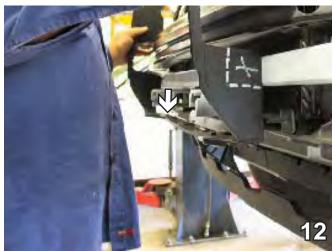
12. Align the air dam as close to the original position as possible, just forward of the baseplate. Mark and trim out area for the air dam and reinstall it to the original position.
