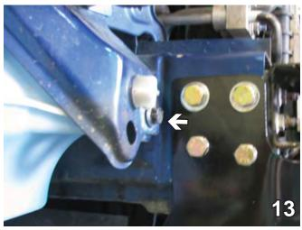
Reinstall the existing metric bolt into the fender support.
