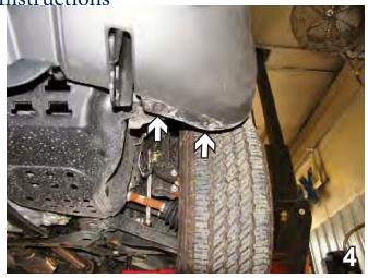
Using a 10MM socket, remove two metric bolts just forward of the front tire, on the bottom edge of the fascia. Do this to both sides of the vehicle. Set bolts aside to be reinstalled later.
