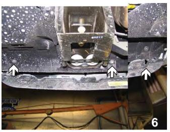
6. Using a 10MM socket, remove three metric bolts from the bottom edge of the fascia. Pull fascia forward and set it aside carefully along with the bolts to be reinstalled later. Some models may need to disconnect electrical plugs from the fog lights.
