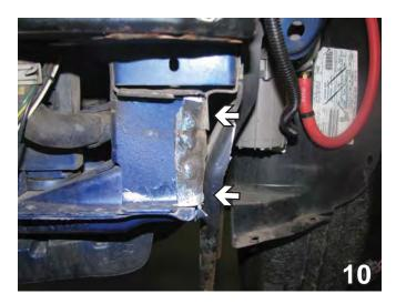
10. Using a pliers, bend over to the inside of the frame. Do this to both sides of the vehicle.
