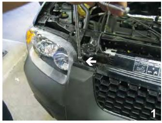
Using a 10MM socket, remove a metric bolt from the top edge of the grill, located just inside head light assembly. Do this to both sides of the vehicle. Set bolts aside to be reinstalled later.
