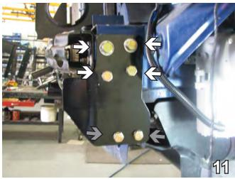
11. Align baseplate with the existing holes of the tie down bracket and insert a 10MMx40MM hex bolt, with a 10MM lock washer and 3/8" flat washer into the top two holes. The middle two holes have a 10MMx40MM hex bolt, with a 10MM lock washer. The bottom two holes have a 10MMx50MM hex bolt, with a 10MM lock washer. Then tighten down using the existing nuts in the frame, with a 13MM socket. Use Loctite Red on all the bolts.\*
