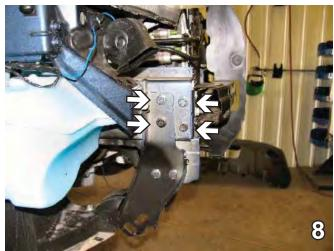
Using a 13MM socket, remove four existing bolts from the tie down bracket. Do this to both sides of the vehicle. The tie down brackets will not be reinstalled.
