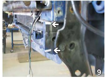
9. Using a reciprocating saw make two slits in the frame. Do this to both sides of the vehicle.
