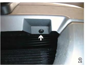
Using a phillips screwdriver, remove a pushpin located just below the license plate. Do this to both sides of the license plate. Set pushpins aside to be reinstalled later.
