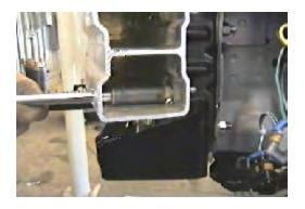
**4.** Remove four metric bolts with 13MM socket from metal bumper and set metal bumper aside.
