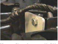
8. Align top of baseplate even with ribbing on top side of frame, as shown in photo, and clamp with vise grips, both sides. Using the baseplate as a template, drill the upper holes with the 13/32" drill bit, both sides.
