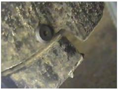
**3.** Just forward of front tires in wheel well, cut two pop rivets with the side cutters, both sides.
