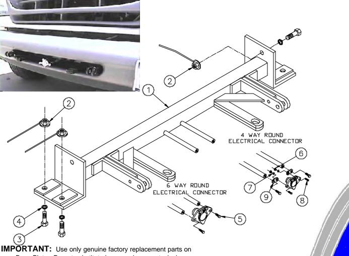
your Base Plate. Do not substitute homemade or nontypical parts. If a bolt is lost or in need of replacement, for your safety and the preservation of your Base Plate, be sure to use a replacement bolt of the same grade (Usually Grade 5, refer to parts list). Repair parts may be ordered through your nearest Blue Ox dealer or distributor.
