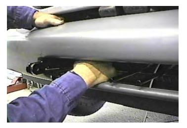
**3.** There are four metric bolts to remove on the metal bumper, using a 21MM socket. Set metal bumper aside.
