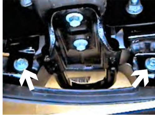
7. Remove two metric bolts from the back side of lower bumper using the 13MM socket. Pull metal bumper forward, disconnect all electrical connections and set metal bumper aside.
