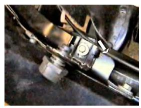
**7.** Using the 10MM socket, remove one metric bolt from hood support guide on both sides, set hood support guide aside.
