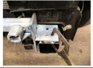
10. Slide baseplate on top of and between frame rails as far back as possible on both sides and clamp in place with the vise grips (Photo to the left). Notice that the base plate is painted white to increase visibility in photos.
