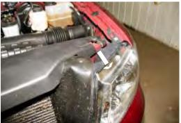
**1.** Remove the push pin from rubber air dam just above headlight assembly, on both sides.
