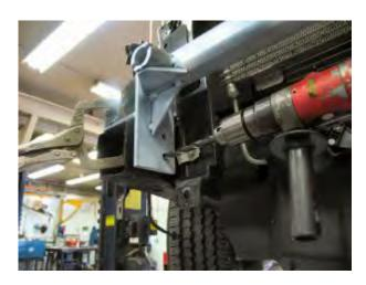
**11.** Using the baseplate as a template, drill two holes on the top and side of frame rail with the 17/32" drill bit, on both sides.
