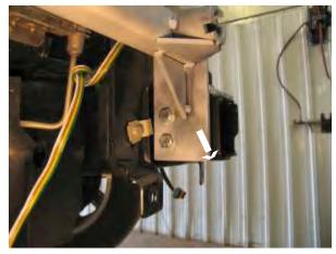
**12.** Insert the 1/2" x 1 1/2" hex bolts into drilled holes on the top side of frame (Left photo), tighten 1/2" lock washers and hex nuts on the inside of frame, on both sides (Photo below). In ert the 1/2" x 1 1/2" hex bolts into drilled holes on the side of frame (Right photo), tighten 1/2" lock washers and hex nuts on the
