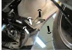
4. Forward of front tires on wheel well edge, are two push pins (White arrows) to remove and two metric bolts (Black arrows) to remove from side panel, with the 10MM socket, on both sides.
