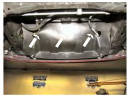
**5.** Remove the three push pins from the lower rubber air dam on bottom edge of fascia.
