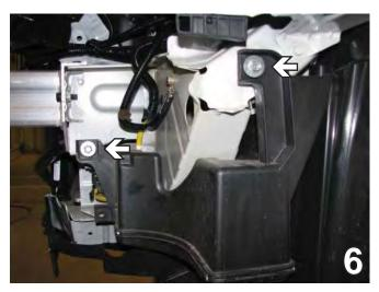
6. On the driver's side, remove the air baffle. Use a 10MM socket to remove the two metric bolts
