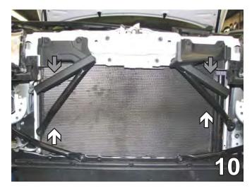
10. If necessary to clear the area for baseplate installation, these plastic braces may be moved out of the way. They just snap on. Be careful not to damage the radiator (gray arrow), then rotate brace out of the way (white arrows).
