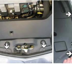
Remove six push pins from the plastic above the radiator, three on each side. Remove the plastic from the top of the radiator. Set pushpins aside to reinstall later.
