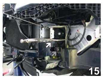
15. Slide the baseplate straight on. Align with the existing lower hole for air baffle on driver's side (gray arrow). Be sure the baseplate is level and clamp with a vise grip. The two lower baseplate holes should align to the middle of doubled lower frame webbing. Using the baseplate as a template, drill the four holes with a 13/32" drill bit. Do this to both sides of the vehicle.
