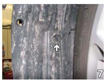
7. On the driver's side only, just forward of the front tire, remove the Christmas tree push pin. Set air baffle and push pin aside to reinstall later.
