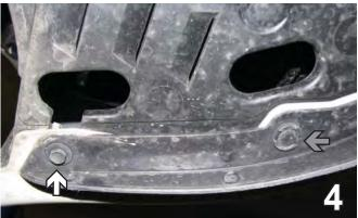
4. Underneath the vehicle along the bottom of the fascia, use a 10MM socket to remove three bolts, white arrows. Also remove the push pin, as indicated by the gray arrow. Do this on both sides of the vehicle. Set bolts and push pins aside to be reinstalled later.
