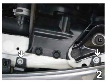
On the top side of the fascia, remove two metric bolts with a 10MM socket. Do this on both sides of the vehicle. Set bolts aside to reinstall later.
