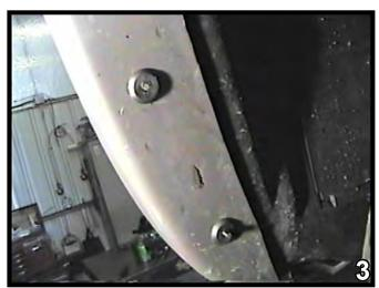
Just forward of the front tire are four rivets, cut and remove the three lower rivets and two rivets on the underside of the fascia corner. Do this to both sides of the vehicle. These rivets will be replaced by others later.
